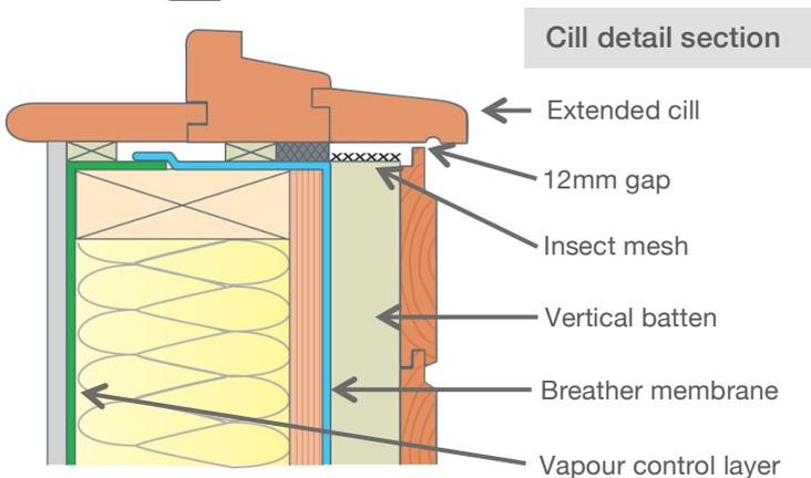
Typical detail of window in horizontal cladding. The drawings show a timber frame wall. Detailing will be similar for other forms of wall construction.
