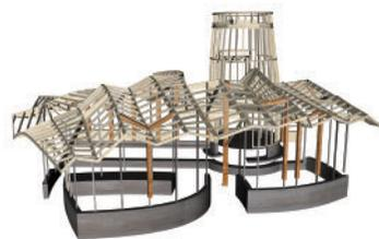
Laminated veneer lumber, or LVL, is typical of the engineered timber solutions made possible by modern manufacturing techniques.
