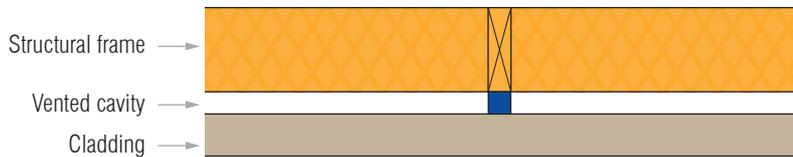
**D6 Plan of vertical cavity barrier**
