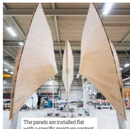
The panels are installed flat with a specific moisture content.
