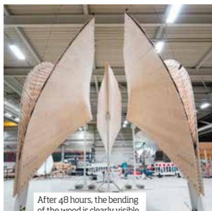
After 48 hours, the bending of the wood is clearly visible.
