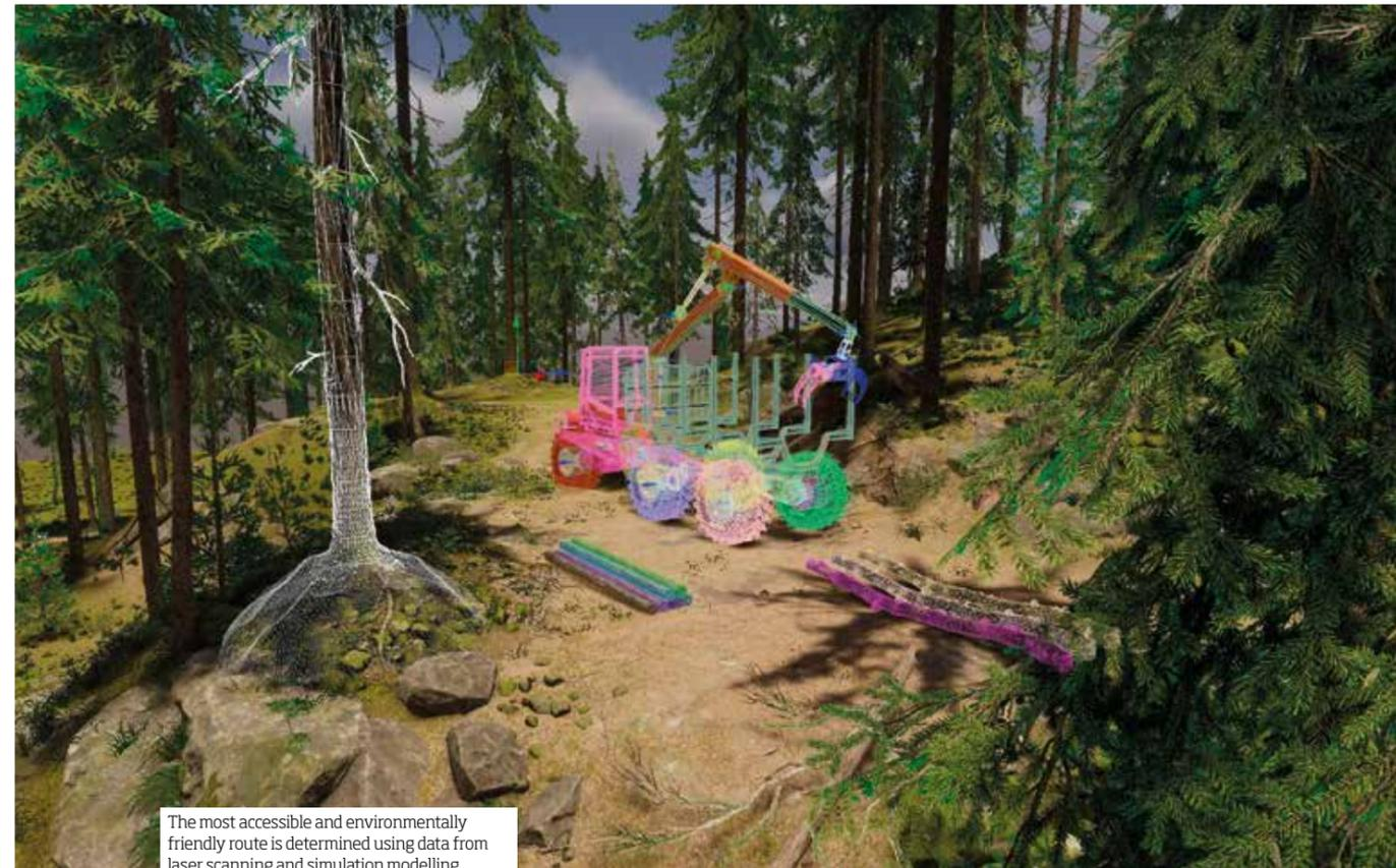
The most accessible and environmentally friendly route is determined using data from laser scanning and simulation modelling.
