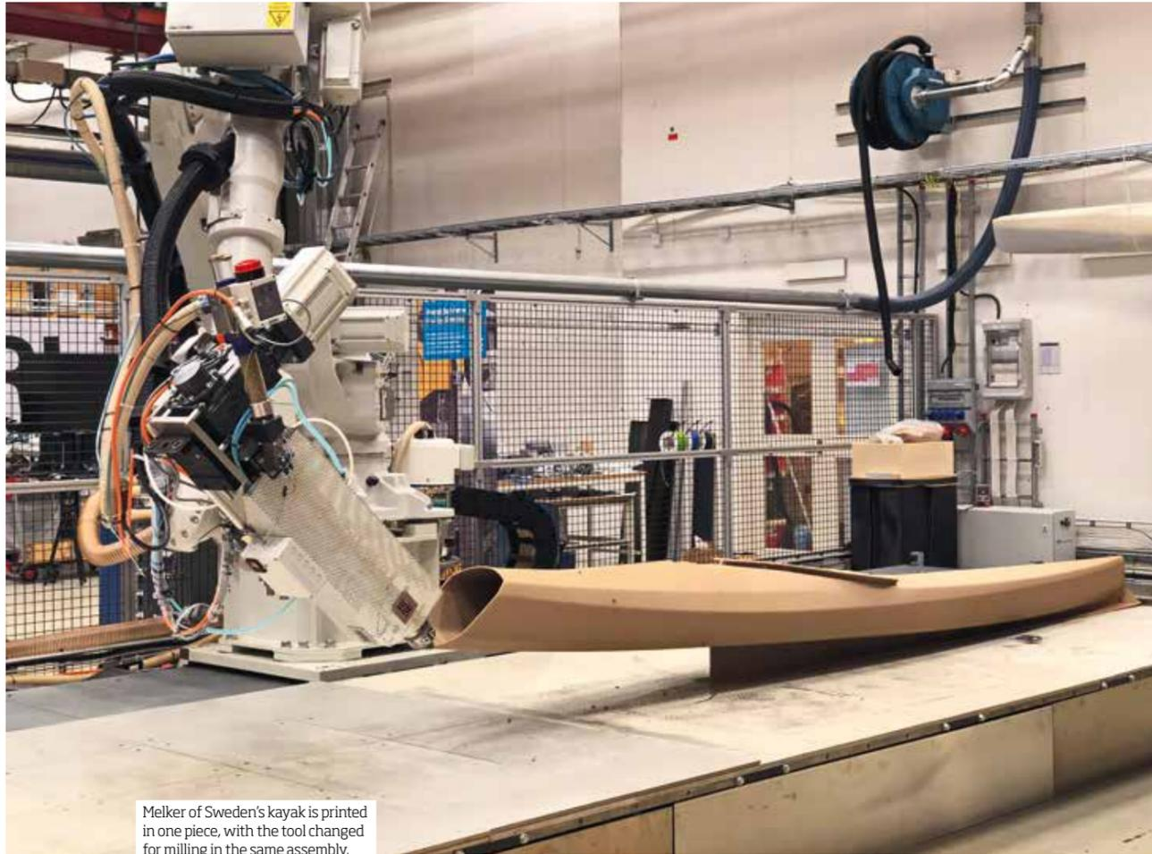
Melker of Sweden's kayak is printed in one piece, with the tool changed for milling in the same assembly.
