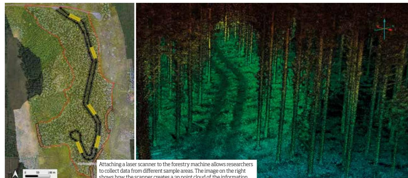
Attaching a laser scanner to the forestry machine allows researchers to collect data from different sample areas. The image on the right shows how the scanner creates a 3D point cloud of the information.
