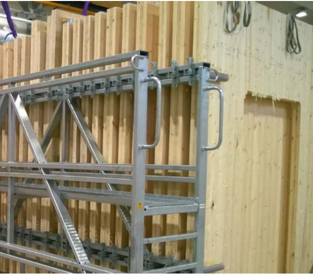
CLT panels ready for supplementary layers.
