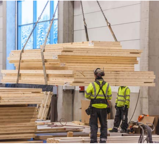
Lifting CLT panels at the factory.
