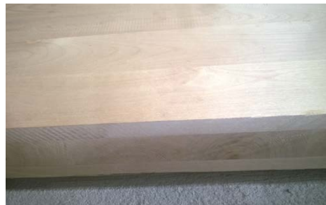
3-layer CLT panel made from birch.
