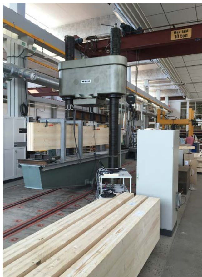
Strength-testing of CLT.
