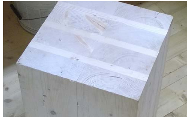
7-layer CLT block made from spruce.
