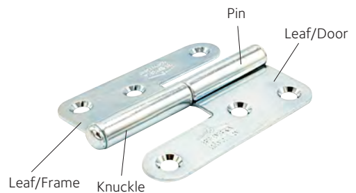
Figure 4.11 Lift off butt hinge
