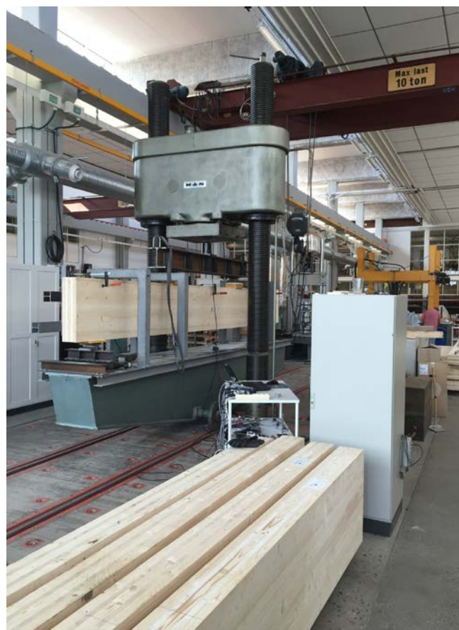
Strength-testing of CLT.
