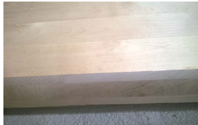
3-layer CLT panel made from birch.
