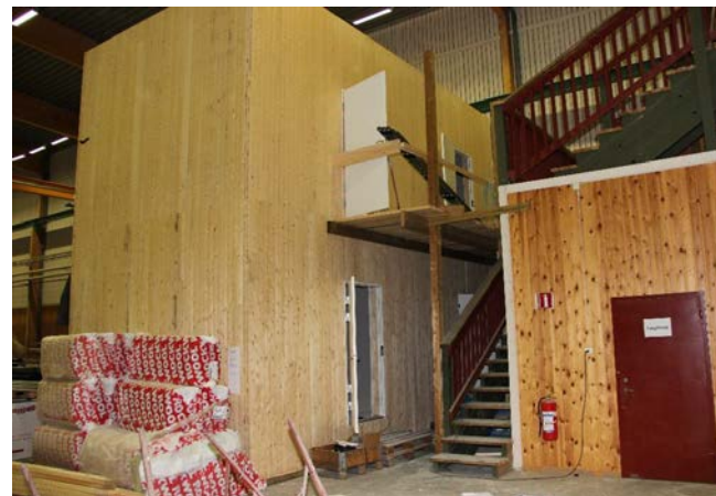
A test house designed for sound measurement, comprising 3 – 4 units.
