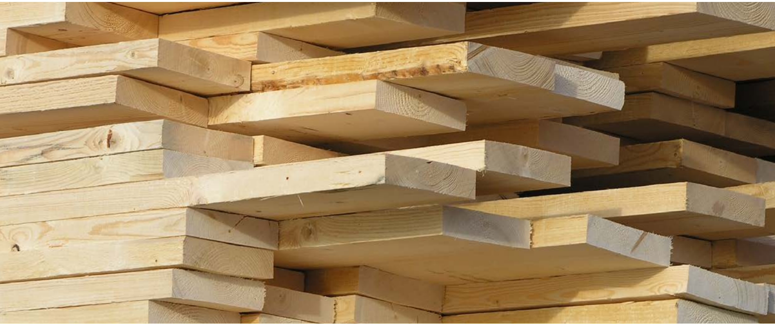
Boards for the production of CLT.
