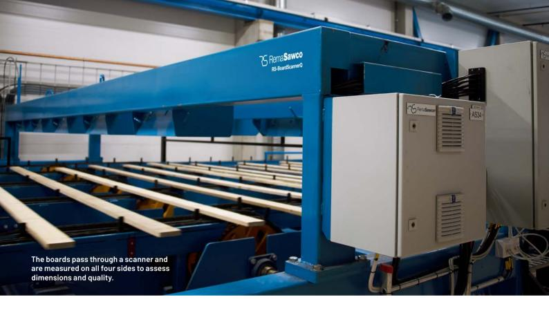
In addition, it is possible to remove pieces of timber that have too high a moisture content.
