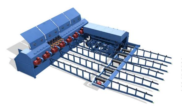
A trimmer consists of a number of blades for modular cutting of timber pieces. The timber pieces are transported through the trimmer on a chain conveyor with carriers and on to the bins.
