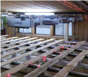
On the green sorting, trimming and planing lines, boards are measured according to customer rules and requirements. Here, a high-resolution 3D laser system is scanning along and across the board to detect geometric defects and then adjust, optimise or classify them.
