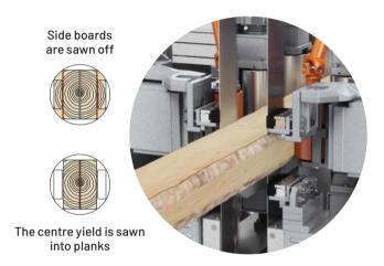
**BAND SAWING** Band sawing of side boards with wane.
