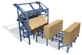
Tilt with extra hoist is used in trimmers and planers. The extra hoist means that no production is lost during package changes.
