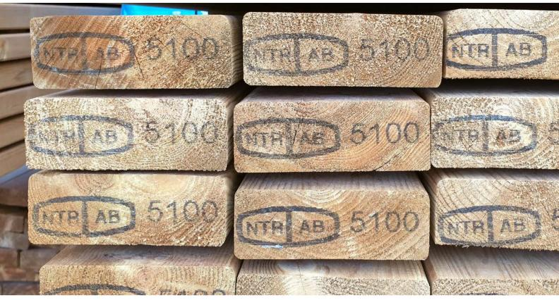
Pressure treated timber must be impregnated in accordance with the regulations of the Nordic Wood Preservation Council, NTR. Wood preservation class NTR AB means that the timber is intended for use above ground, for example for fencing, railings or decking.
