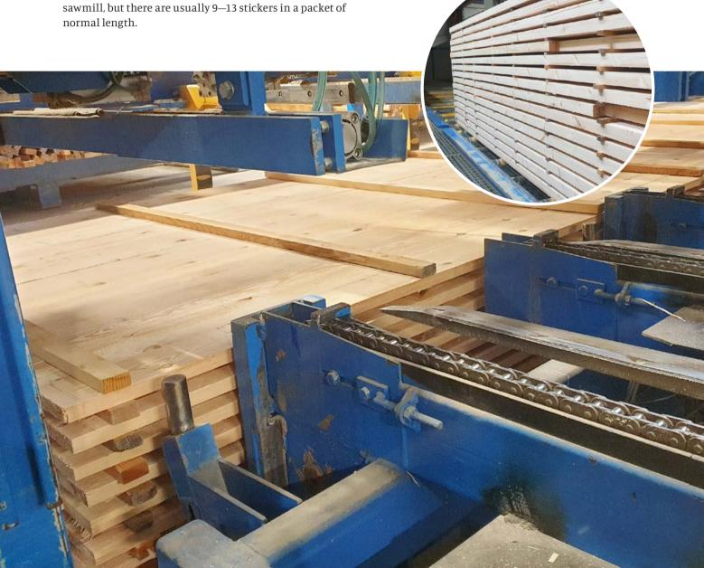
The sticker-stacker builds up packets and places the stickers across the pieces of wood in rows directly above each other. This makes the stacks stable and ensures maximum airflow.
