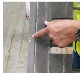
A broken chopping knife can cause poor chip quality.
