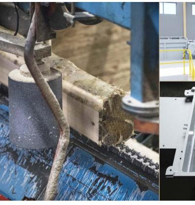
Side board sawing is a first step in the conversion process, where a cant is produced by sawing out two or four boards from both sides of the log.
