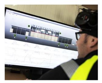
With the help of computers and a number of sensors, the operator can monitor progress in the kiln.
