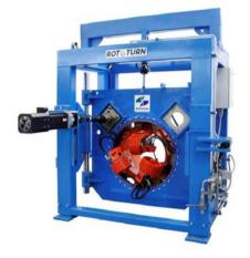
The log rotator accurately rotates the log before centring it in the optimal position for cant sawing as calculated by the measurement and optimisation system.
