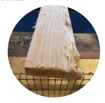
A misaligned board means economic losses, for example in the form of trimmings due to excess wane.
