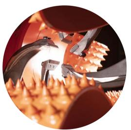
Pneumatically controlled debarking tools with carbide plates.
