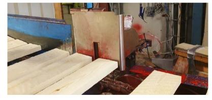
The company's shipping mark is automatically stamped on the end of the timber using a marking device that is permanently installed on the production line.
