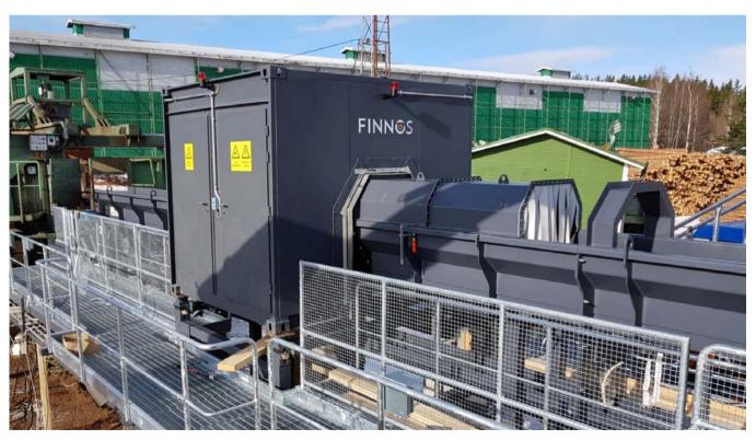
Using x-ray technology, logs can be sorted by internal characteristics at an early stage, ensuring a better yield from the log.
