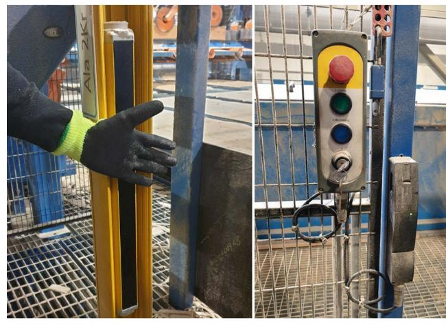
A light barrier or light curtain acts as an invisible fence around a hazardous area to prevent injury. If the light curtain is broken, the machine stops.
