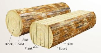
**SAWING, 4EX CENTRE CUT** (Nordic sawing practice)
