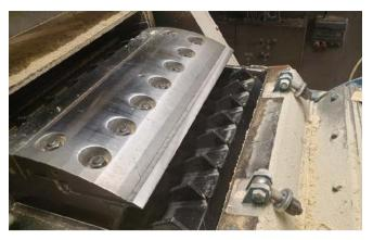
For high-quality cellulose chips, the chipper's cutting tools must be sharp and other machine parts that affect output must be well maintained.
