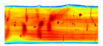
It is of utmost importance to sort out faulty logs before conversion. Logs containing stones, metal and other foreign objects cause production losses during the conversion process.
