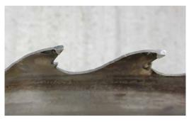
A saw blade with damaged teeth will leave the sawn timber with incorrect dimensions and a defective sawn surface.
