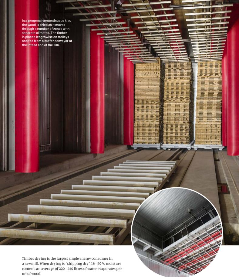
The temperature in Swedish wood kilns is high — between 50 and 80  $^{\circ}$ C — so access to the kiln is highly restricted.
