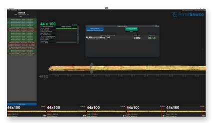
Board optimisation involves assessing the highest value a board can have, given its characteristics and possible cuts.
