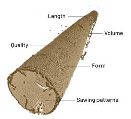
The x-ray frame records all the internal and external characteristics of the log. The recorded information is then used to optimise the sorting for the best value yield.
