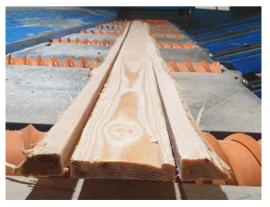
The laths from the edged board are transported to the chipper to be turned into wood chips.
