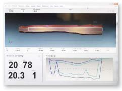
The edger optimises the maximum volume or value of the board based on programmed value data.
