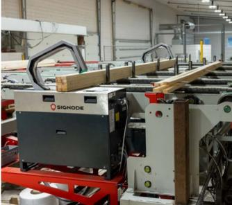
Bundling and strapping of small timber packets is common in the production of smaller dimensions, such as cladding, mouldings and battens.
