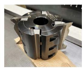
A profile cutter is used to plane cladding and mouldings, but also for custom products.
