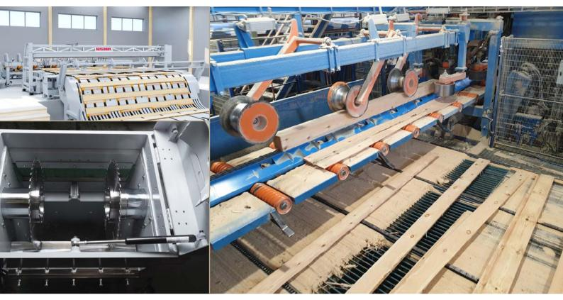
The edger has two parallel blades that can be quickly positioned at high feed rates.
