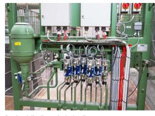
Sectional distributor for hydraulic pressure to the various components of the machine equipment. The distributor is located close to each machine group for easy access and ensures precise control and monitoring of the hydraulic flow directly alongside the saw line.
