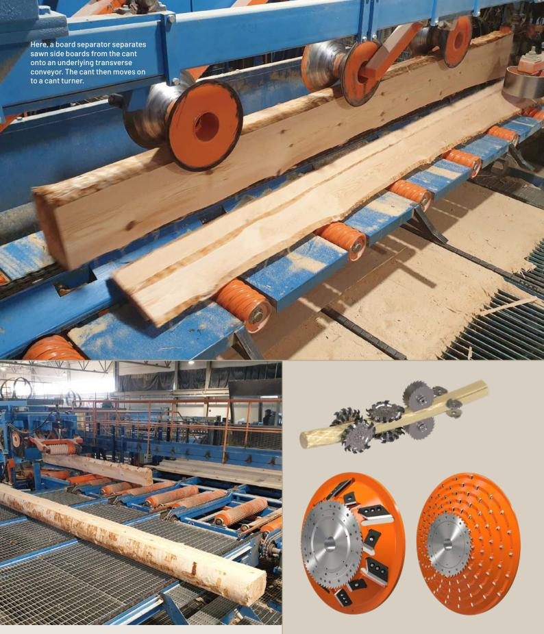
Saw line for different sized logs with features such as optimisation, curve sawing, edging, high-speed infeed and quick change of sawing pattern.
