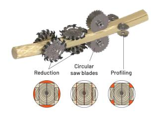
Reducing, breaking down and profiling in the same machine.
