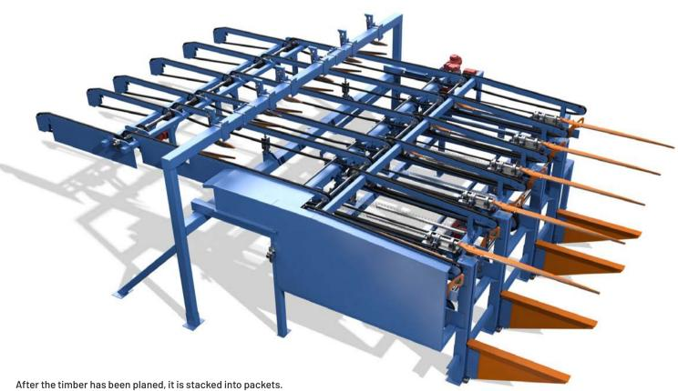
A stacker is capable of forming all kinds of packets, such as full, half and quarter packets. Binding sticks are placed in the packet between predetermined layers and loaded manually into a cassette on the walkway next to the machine.
