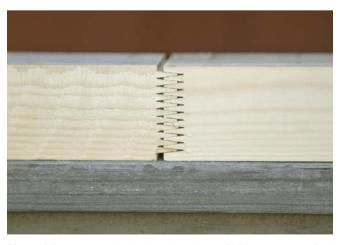
Finger-joints are used when lengths of over 5400 mm are required.
