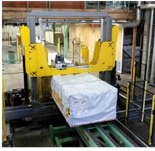
Fully automated polyester strapping machine with electric top and side press.
