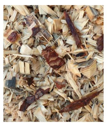
Bark and contaminants must not be present in wood chips destined for pulp and paper production.
