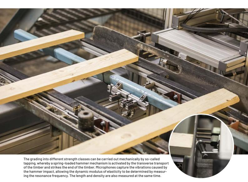
Strength grading of construction timber for load-bearing structures usually takes place mechanically or visually. The old visual grading rules (T-virkesreglerna) have been replaced by joint Nordic grading regulations. In Sweden they are issued as Swedish standard SS 230120, while the joint Nordic designation is INSTA 142. The rules apply to pine, spruce, silver spruce, larch, Sitka spruce and Douglas fir. The wood continues to be called T-virke and the classes are T0, T1, T2 and T3.
