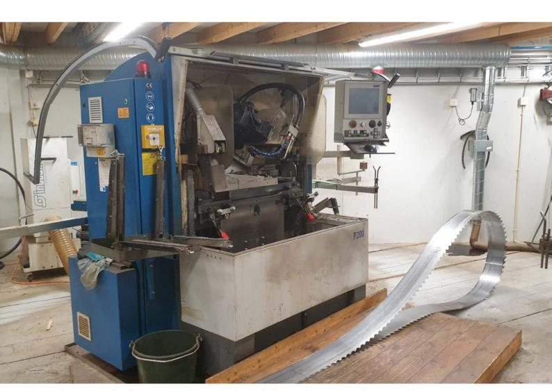
Sharpening saw blades is an important part of saw production. A grinding machine must be kept in good condition to ensure the right dimensions of the timber and a good sawn surface. It will also make saw blades last longer with more efficient sawing.
