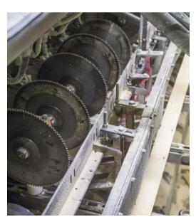
A trimmer has a number of blades for cutting lengths of wood. Each piece is transported through the trimmer on a chain conveyor and cut to the desired length.
