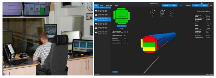
The sawmill operator uses a number of screens to monitor production on the saw line and can study the optimisation software's assessment of each individual log.
