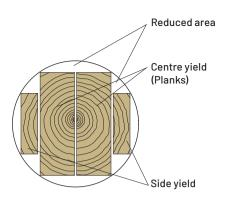
After reduction, the cant can be broken down in different ways.
