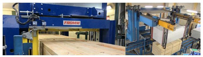
Automated machine for polyester (PET) strapping, together with a press that compresses the packets during strapping.
