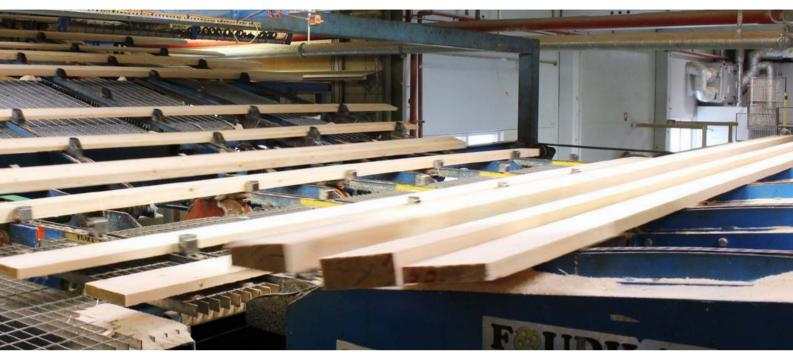
After conversion, all the wood is checked before being sorted into different dimensions.
