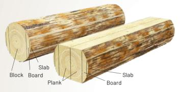
SAWING, 2EX CENTRE CUT (Nordic sawing practice)
