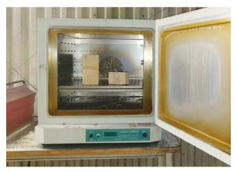
Using a drying cabinet, the moisture content of wood can be calculated with great accuracy by the oven dry method.
