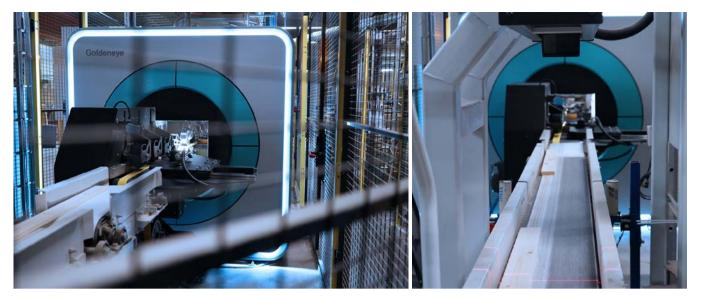
Timber quality can be scanned automatically using x-rays, cameras and sensors. The camera technology determines the characteristics of the timber and is able to locate different types of knots, cracks, discolouration and so on, to determine the true value of each individual board or plank.
