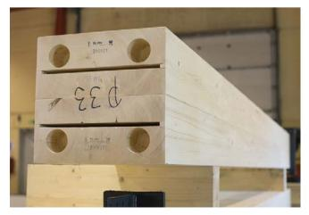
A wooden component that has been industrially drilled and grooved ready for fixings.
