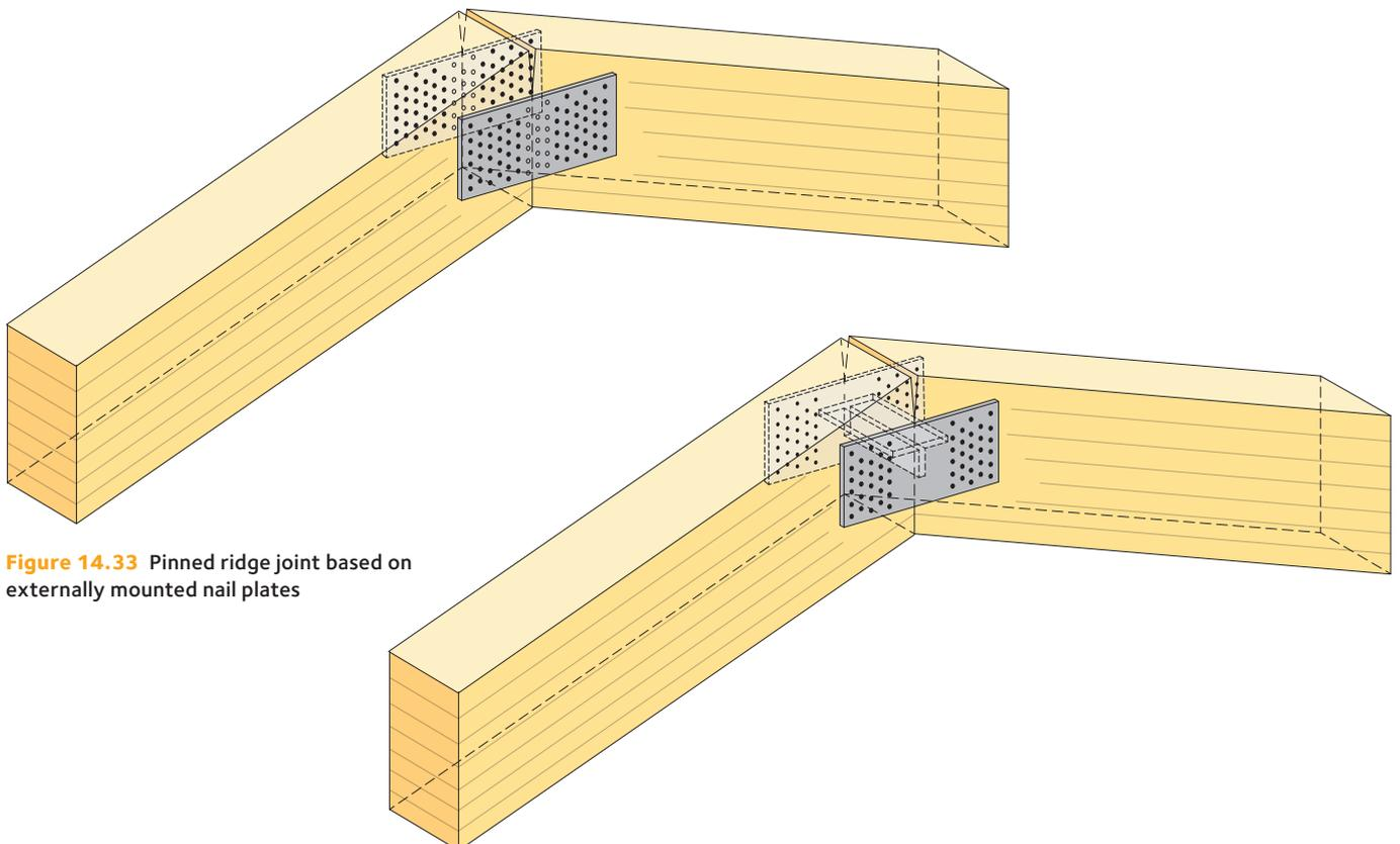
**Figure 14.33** Pinned ridge joint based on externally mounted nail plates
