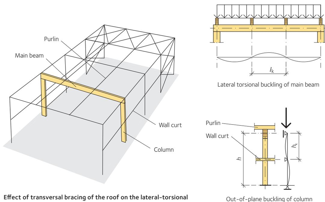
**Figure 13.12** Effect of transversal bracing of the roof on the lateral-torsional buckling of a main beam and on the out-of-plane buckling of a column
