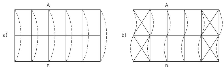
**Figure 4.6** Lateral buckling of a roof or floor system
