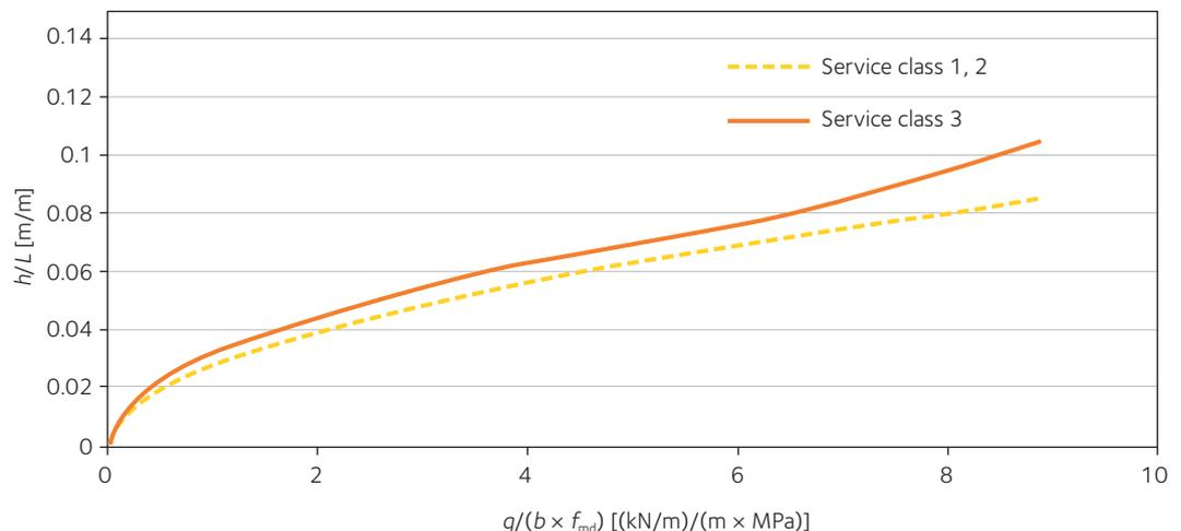
**Figure 4.1** Necessary beam sizes expressed as beam depth/span ratios for varying load levels. Calculated for service classes 1, 2 and 3 respectively using GL30c.  $f_{md}$  calculated according to equation 2.9. Design criteria used are related to the bending stress and shear stress (including  $k_{cr} = 0.85$ ). Beams have to be prevented from lateral buckling.
