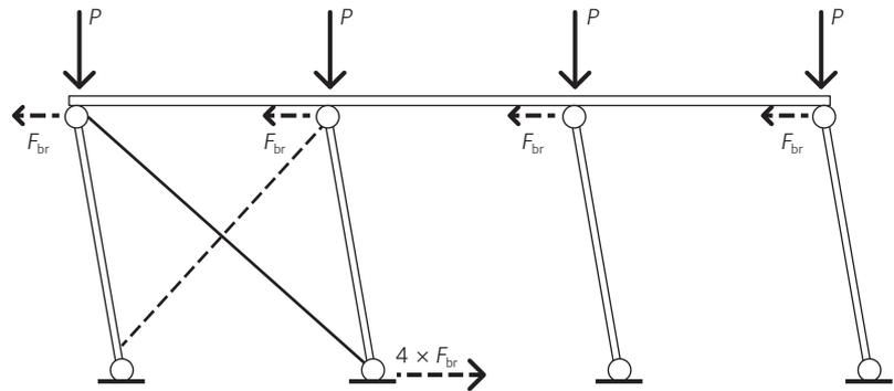
Figure 13.36 Brace force generated by the out-of-plumb of the columns
