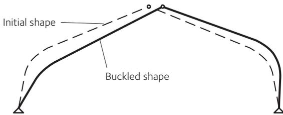
**Figure 10.7** In-plane buckling of a three-hinged portal frame
