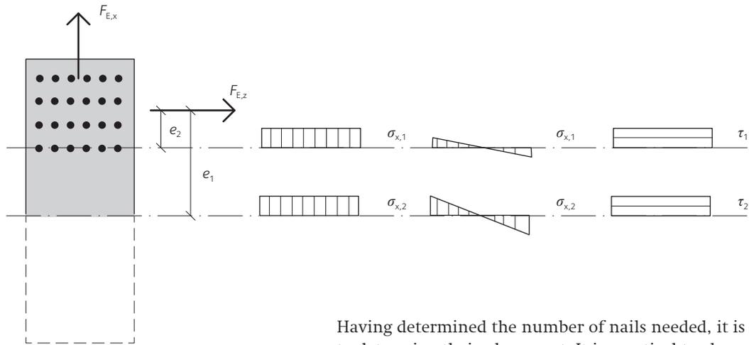
**Figure 14.11** Stress distribution in the steel plate
