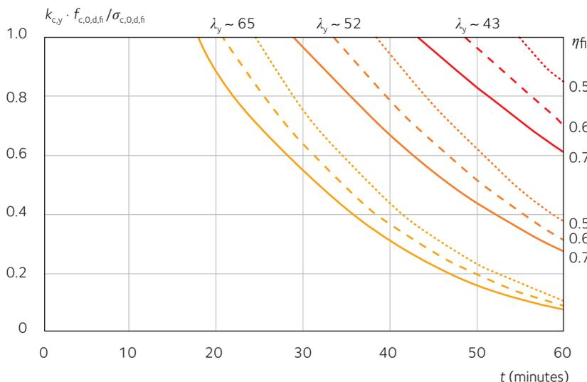
**Figure 16.21** Fire resistance of glulam columns with different slenderness ratios
