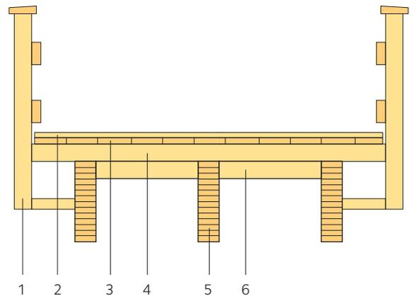
**Figure 3.24** Girder bridge with transverse secondary beams and planks. 1) Handrail, 2) road surface, 3) planks, 4) transverse secondary beam, 5) glulam beams, 6) wind bracing.
