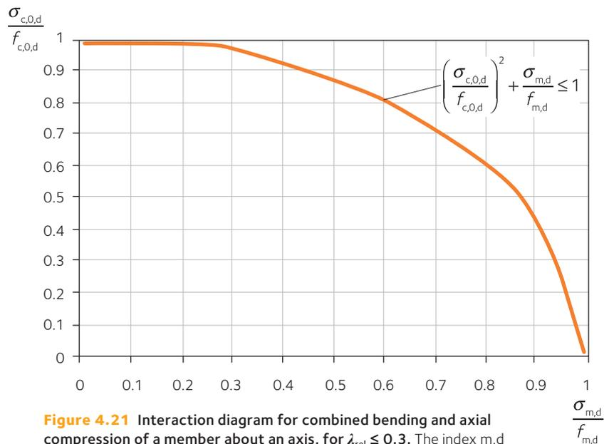
**Figure 4.21** Interaction diagram for combined bending and axial compression of a member about an axis, for  $\lambda_{rel} \leq 0.3$ . The index m,d is used as a generic and refers to bending stress and bending strength respectively, caused by a bending moment either around “y” or around “z”. The index c,0,d refers to axial compression.
