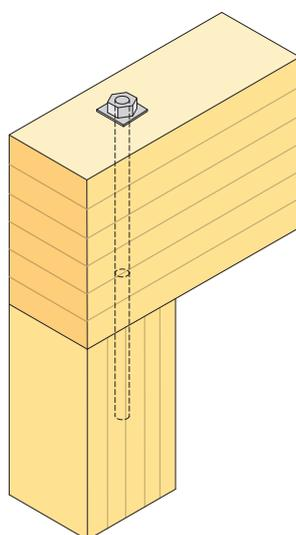
**Figure 14.29** Column top with a bonded-in rod
