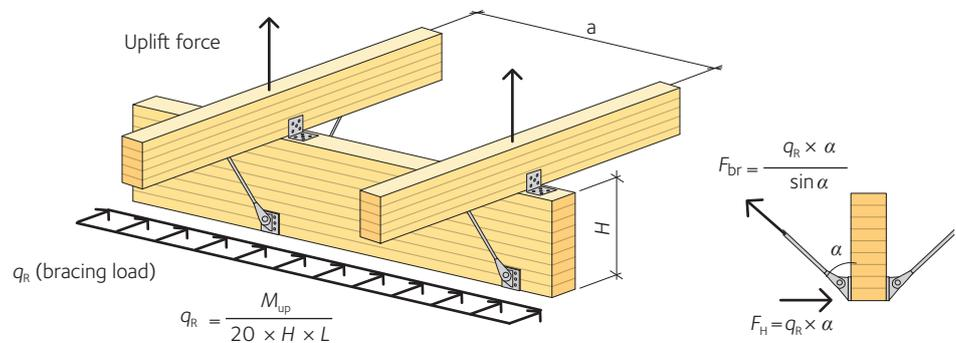
**Figure 13.47** Model for the estimation of the bracing force in the steel rods
