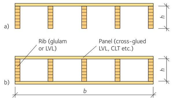
**Figure 13.30** Typical cross-section of wood-based roof systems
