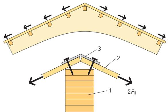
**Figure 12.6** Inclined roof with purlins and roof sheathing
