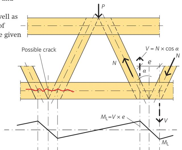
**Figure 8.11** Bad example of truss with eccentricities at the nodes. In the figure, the diagram of eccentricity moments and a possible crack location due to tension perpendicular to the grain are also indicated.
