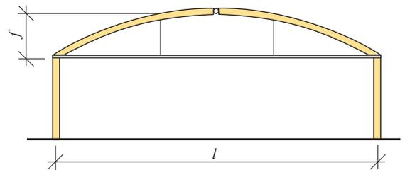
**Figure 11.1** Arch with tension tie, on columns
