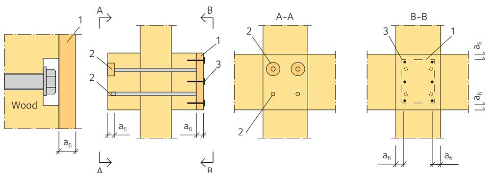
Figure 16.13 Protections for bolts and dowels
