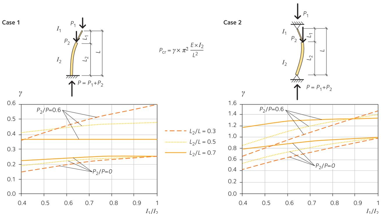
**Figure 4.15**  $\gamma$  factor for determining the buckling load of stepped columns with two different cross-sections and subjected to non-uniform compressive load. Case 1 (left): Cantilever column. Case 2 (right): column with pinned ends.
