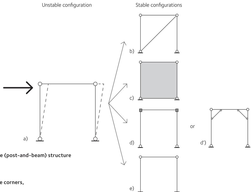
**Figure 13.1** a) Conversion of an unstable (post-and-beam) structure into a stable structure by means of:
