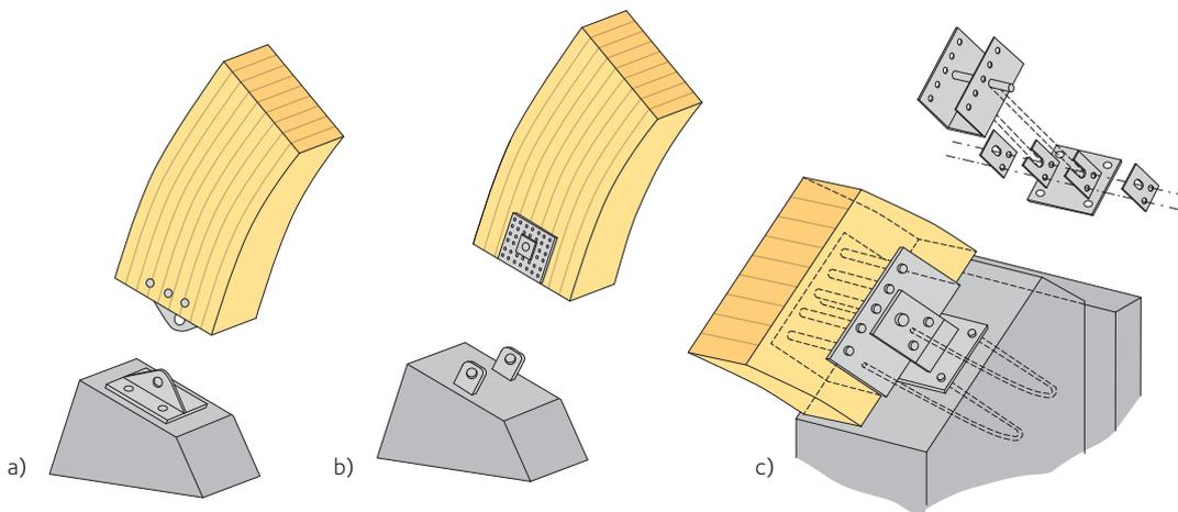
Figure 11.16 Possible arch base details of arches
