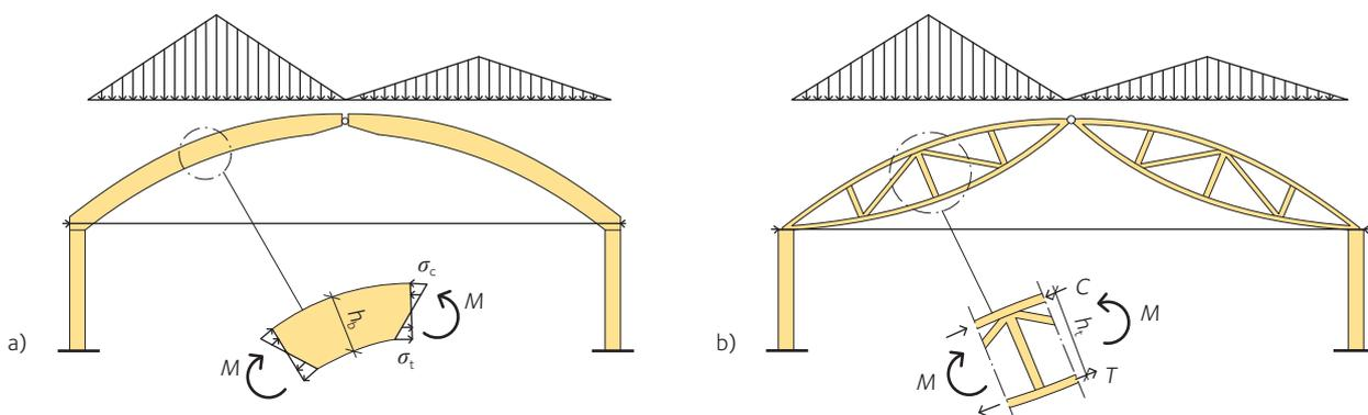
**Figure 11.4** Arch structures subjected to triangular load distribution
