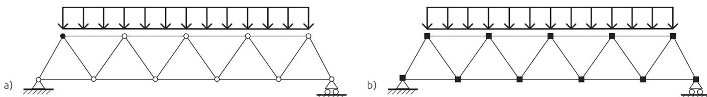
**Figure 8.14** Static system that should be analysed for the determination of bounds for the forces and moments in the members. Both trusses have continuous top chord and bottom chord. a) Truss with hinged web members, b) truss with moment stiff web members.
