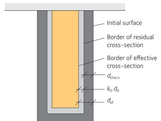
**Figure 16.7** Residual and effective cross-section according to EN 1995-1-2
