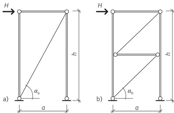
**Figure 13.16** Model for estimation of lateral stiffness of a bay braced by diagonals
