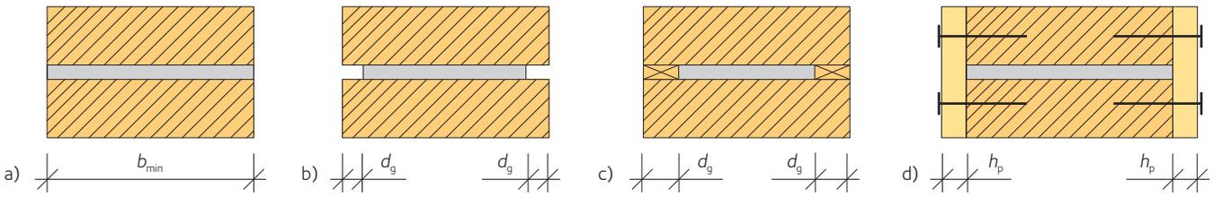
**Figure 16.14** Edge protection for steel plates inside wood
