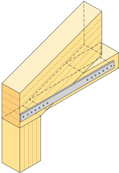
**Figure 14.35** Tie made from glulam with nail plate to transfer the load at its end
