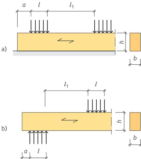
**Figure 4.10** Member loaded in compression perpendicular to the grain, placed on a continuous support a) or on discrete supports b).
