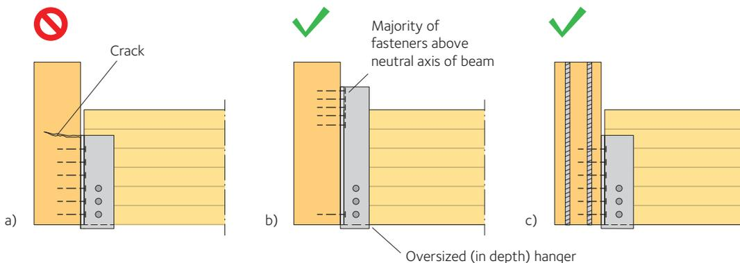
**Figure 15.6** Primary beam to secondary beam connections
