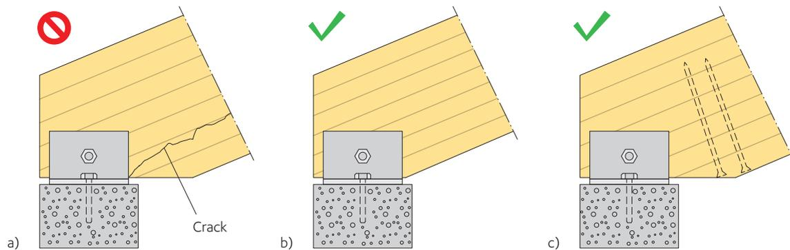
**Figure 15.3** Supports of inclined beam member or arch
