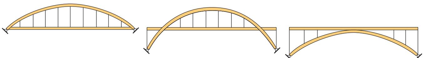
**Figure 3.25** Arch bridges with through, half-through and top roadways
