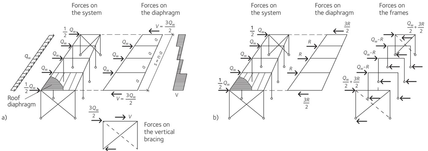
**Figure 13.27** Load sharing mechanisms
