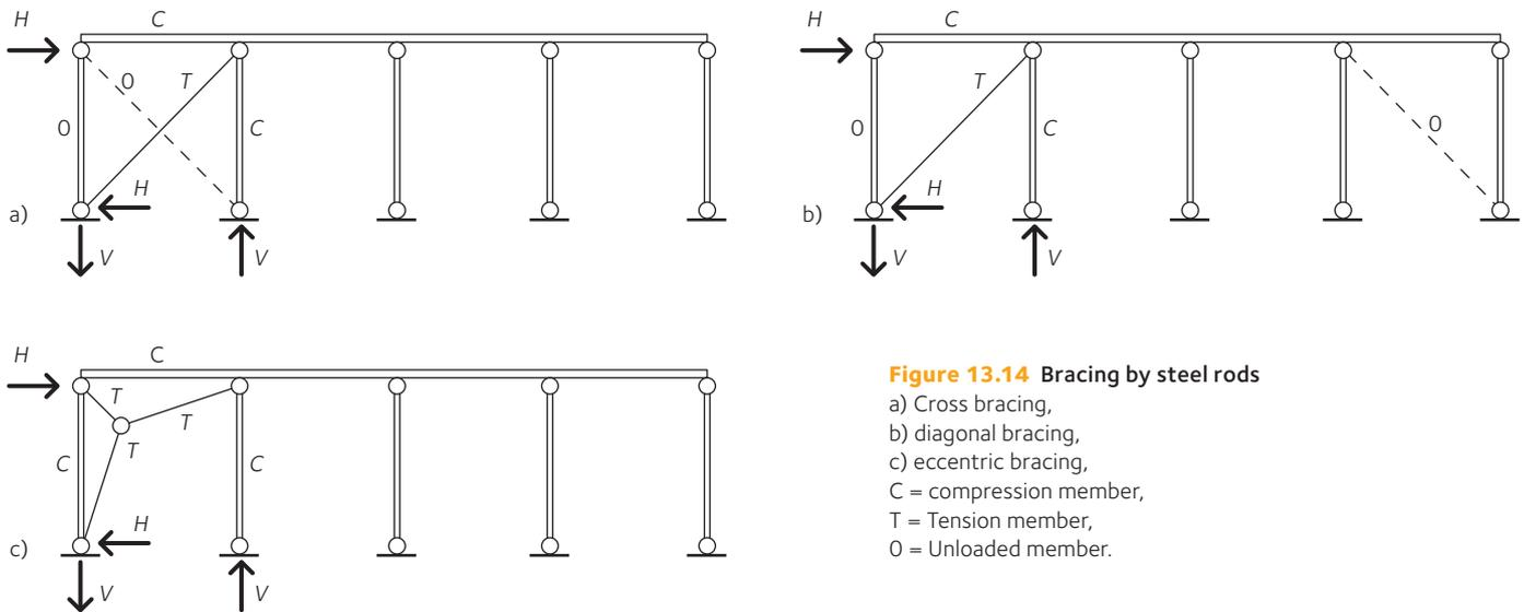
**Figure 13.14** Bracing by steel rods
