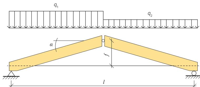
**Figure 9.3** Three-hinged truss with two rafters and tension member (tie) subjected to gravity loads
