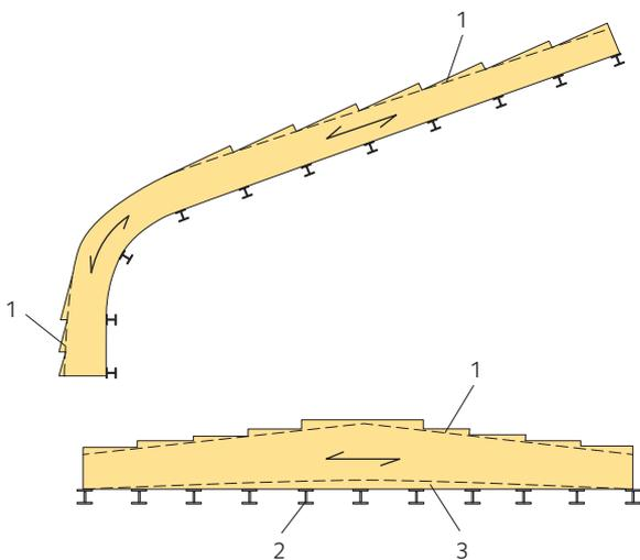
**Figure 1.5** Structural component with varying sectional height
