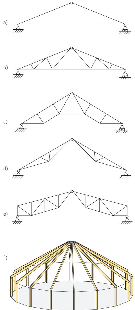
**Figure 3.9** Three-pin trusses
