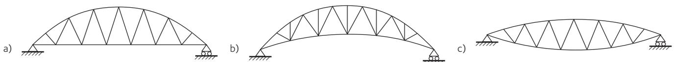
**Figure 8.5** Examples of bowstring and lenticular trusses
