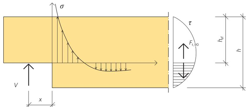
**Figure 5.2** Schematic illustration of stress distribution at notch corner and illustration of tensile force resultant  $F_{t,90}$
