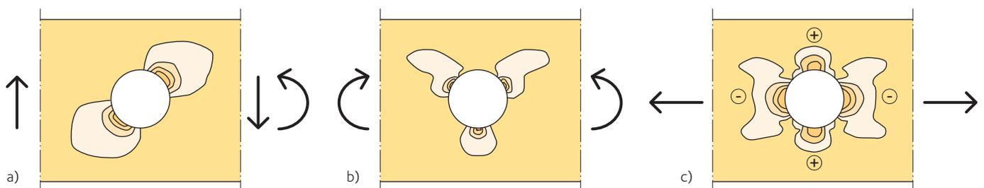
**Figure 5.4** Schematic illustrations of perpendicular to grain tensile stress distribution
