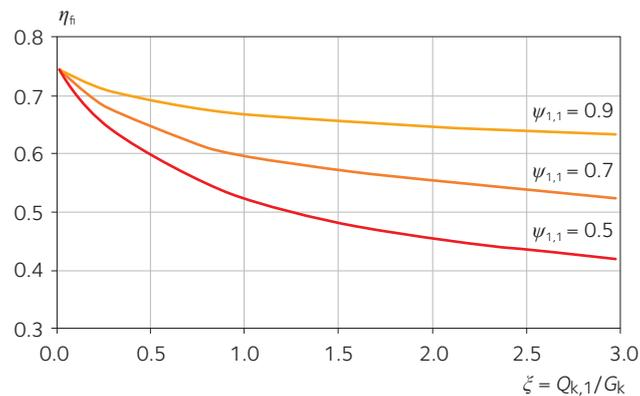
Figure 16.6 Values for  $\eta_{fi}$  as a function of permanent/variable actions ratio  $\xi$
