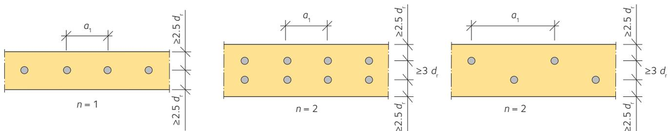
**Figure 7.21** Definition of "n" and  $a_1$  in *equation 7.26* and *equation 7.27* ("n" is the number of groups of reinforcement bars in the direction perpendicular to the longitudinal axis of the beam).  $d_r$  is the outer thread diameter of the reinforcement.
