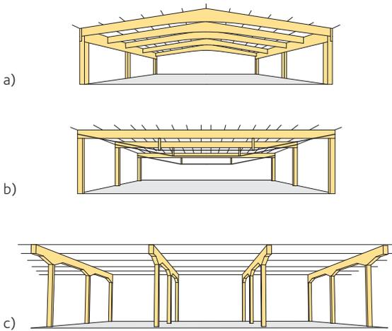
**Figure 3.4** Beam and column system
