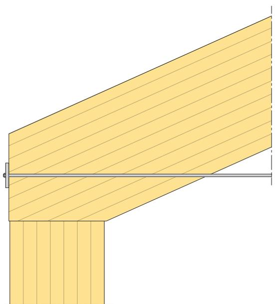
**Figure 16.33** Steel tension tie fixing: Requires fireproofing
