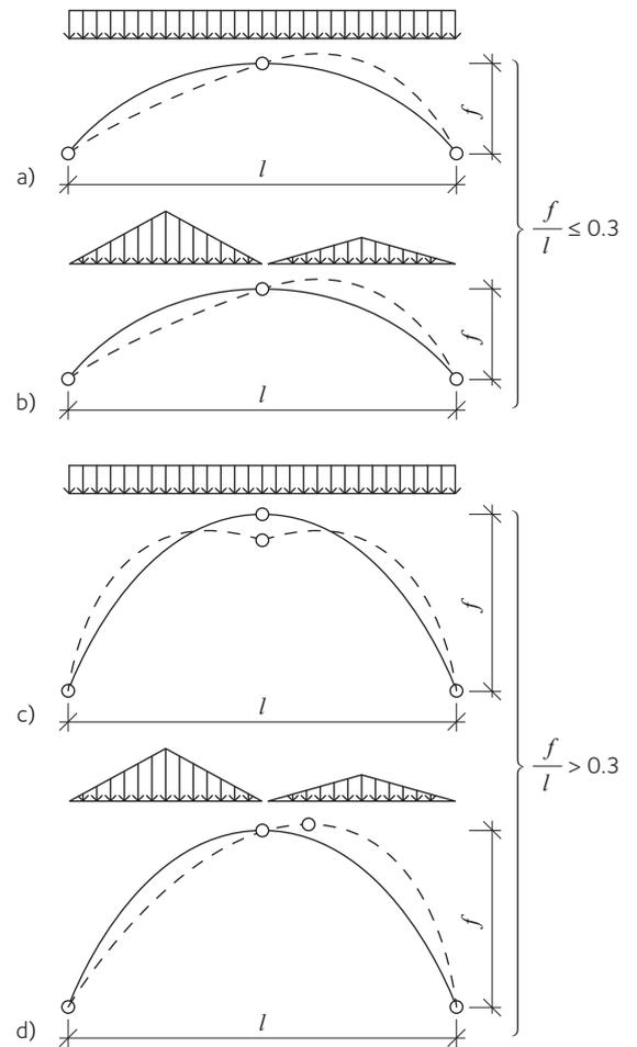
**Figure 11.12** In-plane buckling of three-hinged arches
