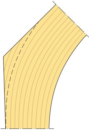
Figure 10.10 Curved haunch with fully glued corner piece
