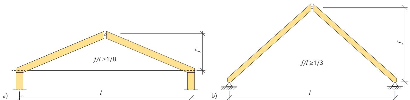
**Figure 9.1** Three-hinged trusses
