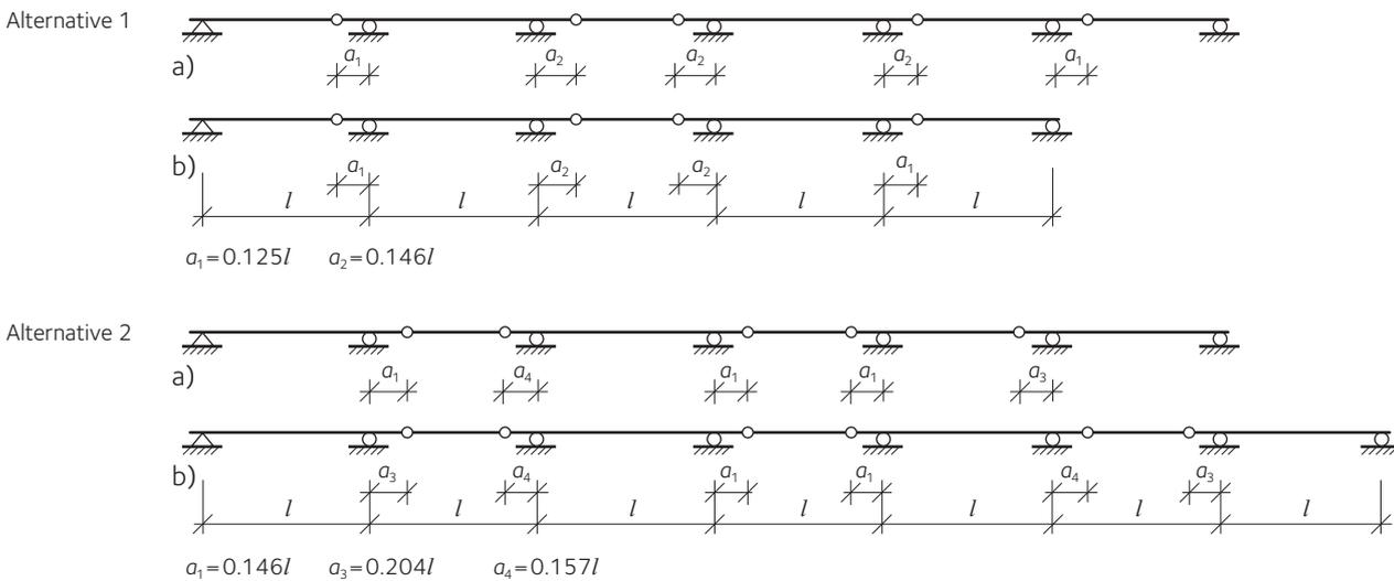
**Figure 12.4** Various types of Gerber systems. Alternative 1: Joint in end bay. a) Even number of bays, b) odd number of bays. Alternative 2: End bays without joints. a) Even number of bays, b) odd number of bays.
