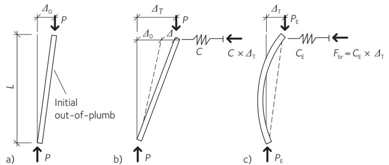
Figure 13.37 Relative bracing system
