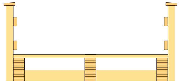
**Figure 3.23** Girder bridge with planks laid directly on the glulam beams
