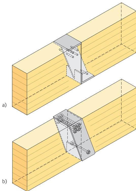
**Figure 14.31** Gerber joints with
