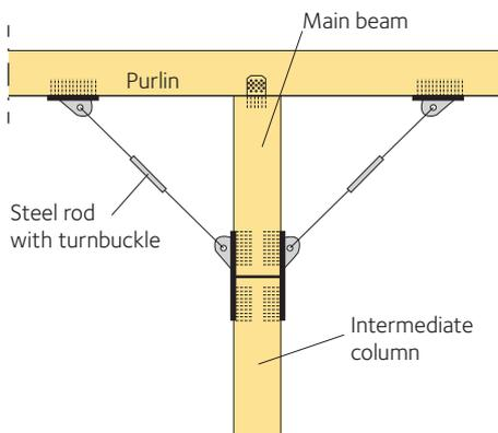
**Figure 4.5** Lateral bracing of a slender beam at lower edge – above intermediate support – connected to roof structure. This bracing should not be able to take compressive forces. For non-symmetrical loading on the roof, which induces deflection of the roof on one side of the beam, and if the bracing can take compressive forces, then the bracing could push the beam over and lead to lateral buckling.
