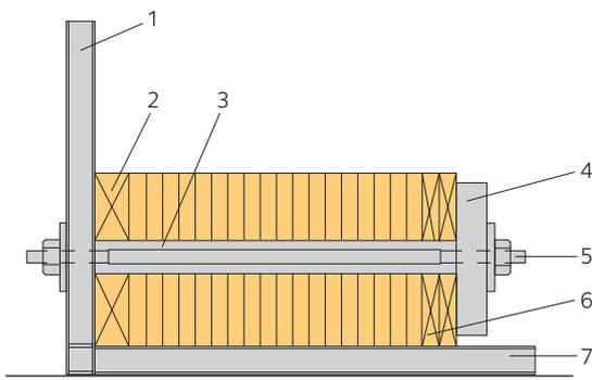
**Figure 1.4** Schematic section through gluing bench
