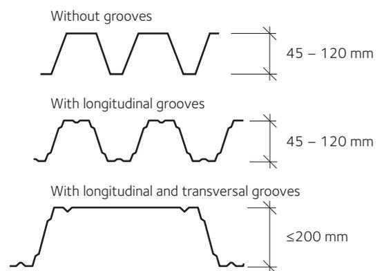
**Figure 13.31** Typical cross-section of trapezoidal metal sheeting
