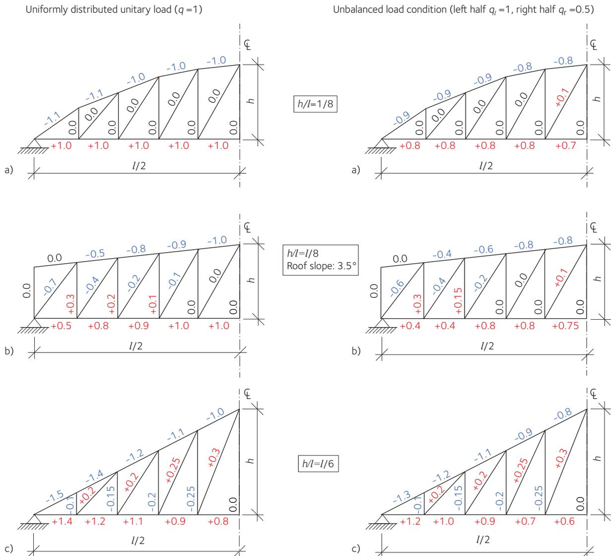
**Figure 8.6** Magnitude of normal forces in three different truss types: a) Bowstring, b) pitched trapezoidal and c) pitched triangular (bottom). Left: uniformly distributed unitary load ( $q = 1$ ). Right: unbalanced load ( $q_l = 1$  on the left half span and  $q_r = 0.5$  on the right half span).
