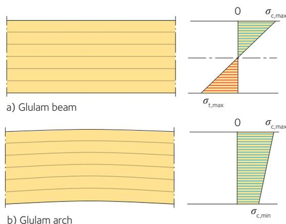
**Figure 3.15** Bending stresses in a loaded beam a) vary through the depth. Compression at the top and tension at the bottom. At the centre of the cross section the stress is zero. An arch b) on the other hand has compression throughout its cross-section.
