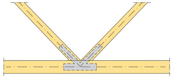
**Figure 14.38** Truss joint based on slotted-in steel plates
