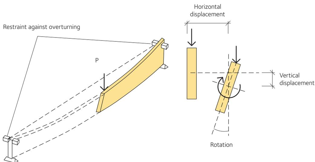
**Figure 4.2** Lateral-torsional buckling of a simply supported beam
