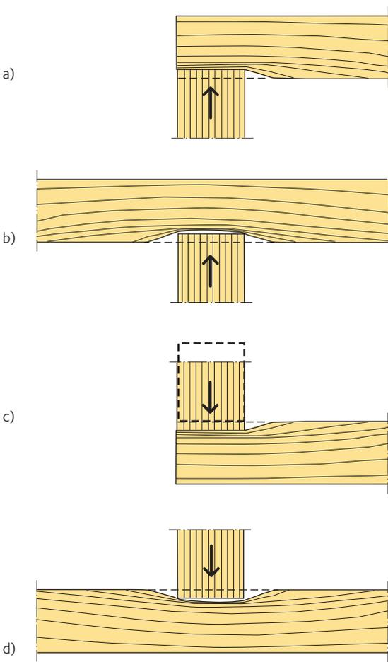
**Figure 4.7** Bearing failure perpendicular to the grain
