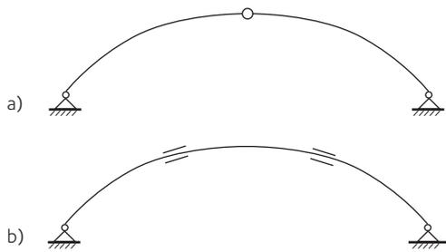
**Figure 11.3** Suitable placing of joints in arch structures
