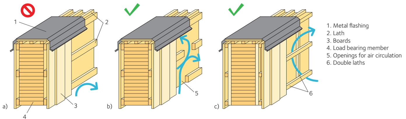
**Figure 15.12** Protection of load-bearing members
