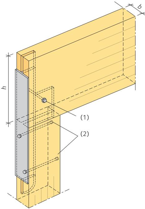
**Figure 16.26** Column-beam connection with slotted-in T-profile: R30 or R60 depending on dimensions
