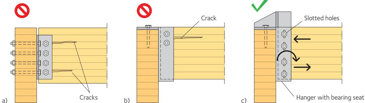
**Figure 15.9** Beam-to-beam connections
