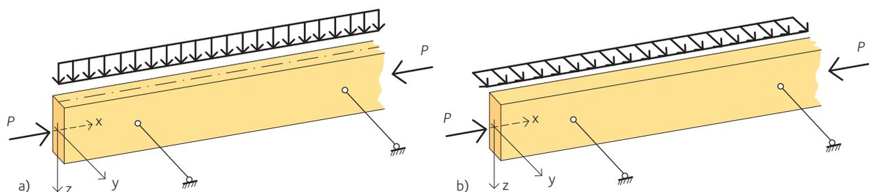
**Figure 4.20** Interaction bending and axial force
