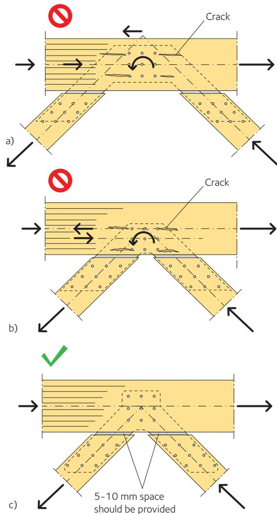
**Figure 15.4** Truss nodes with slotted-in plates and dowels
