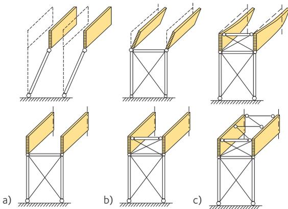
**Figure 13.3** Stabilization of a bay of a structure
