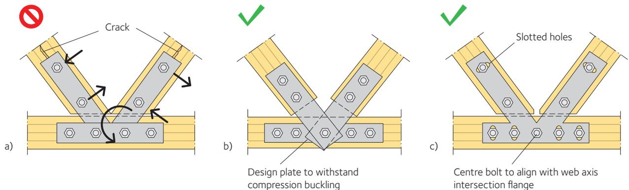
**Figure 15.5** Truss nodes with external plates and bolts
