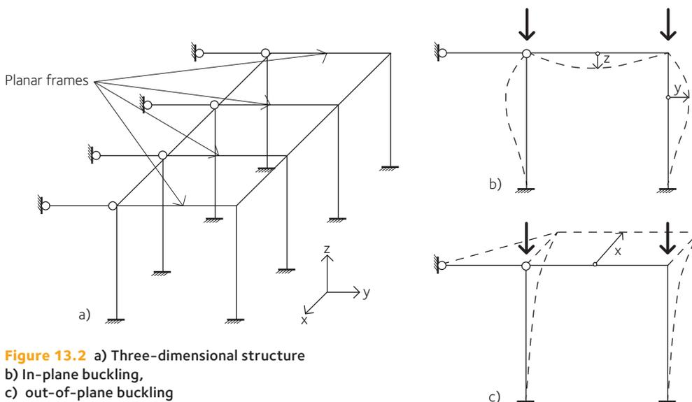
**Figure 13.2** a) Three-dimensional structure
