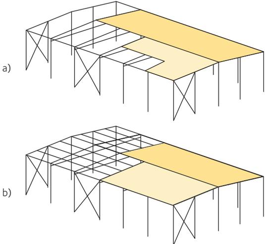
**Figure 13.28** Roof diaphragm arrangements
