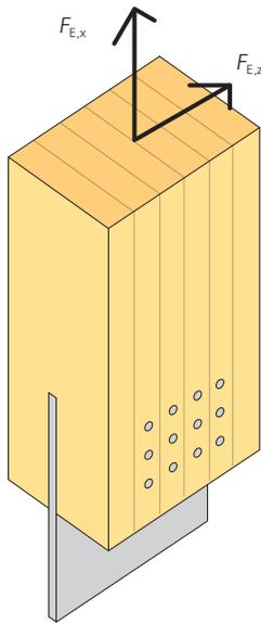
**Figure 14.13** Slotted-in steel plate for pinned column base
