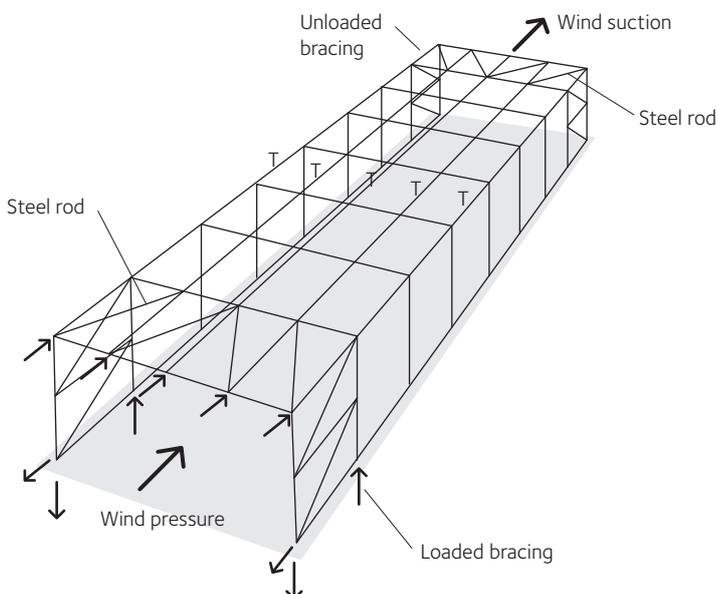
**Figure 13.24** Example bracing systems with only one steel diagonal in each web panel. Such a system is “unidirectional”, which means that it can only work if the load is applied in the direction that causes tension in the diagonals.
