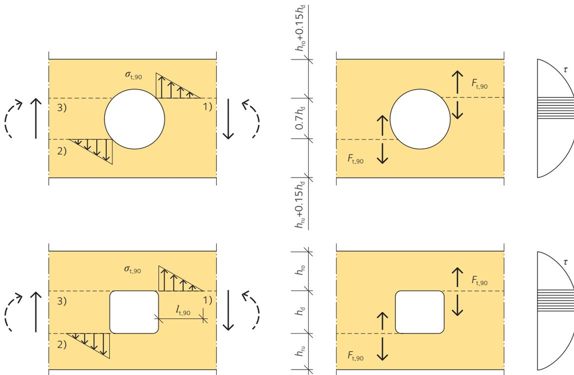
**Figure 5.6** Location of critical planes concerning cracking for rectangular and circular holes
