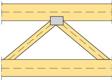
**Figure 14.2** A joint which is placed eccentrically in relation to system lines (dashed lines)
