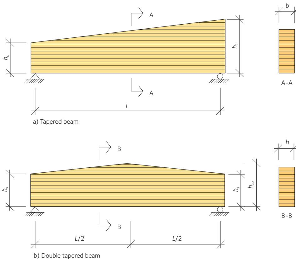
Figure 6.4 Tapered beams
