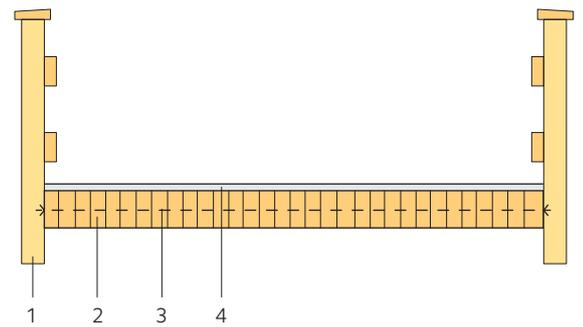
**Figure 3.22** Slab bridge with transversely pre-stressed slab of glulam. 1) Handrail, 2) upright glulam beams, 3) steel tension rod, 4) road surface.
