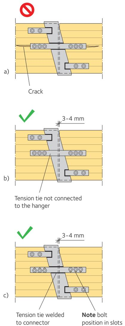
**Figure 15.8** Gerber type hangers with tension-tie
