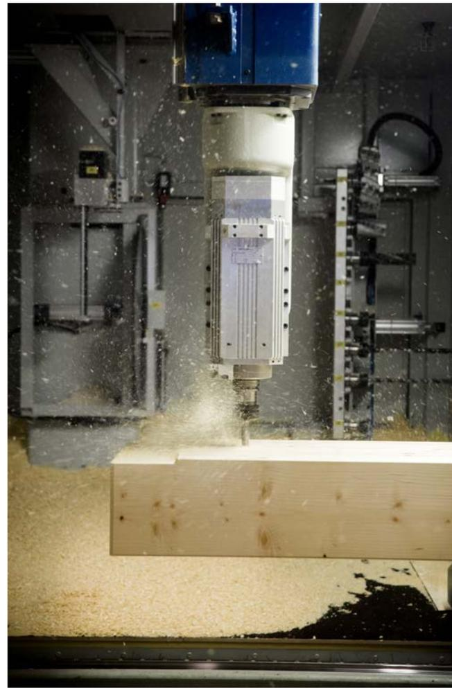
CNC machining of glulam beam.
