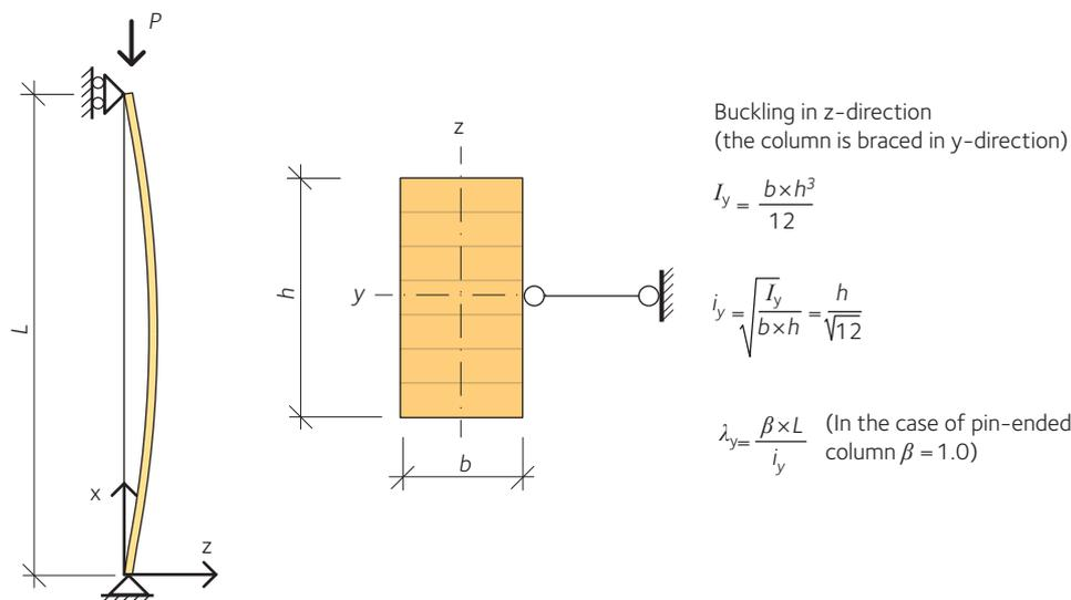
**Figure 4.17** Buckling of a timber column: definition of moment of inertia ( $I$ ), radius of gyration ( $i$ ), and column slenderness ( $\lambda$ )
