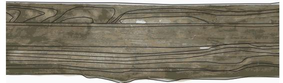
**Figure 16.2** Glulam beam without significant singularities after a fire
