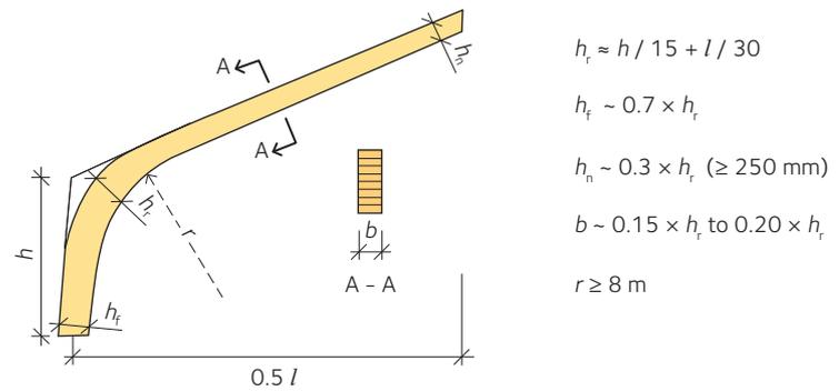
**Figure 10.3** Preliminary sizing of a glulam portal frame
