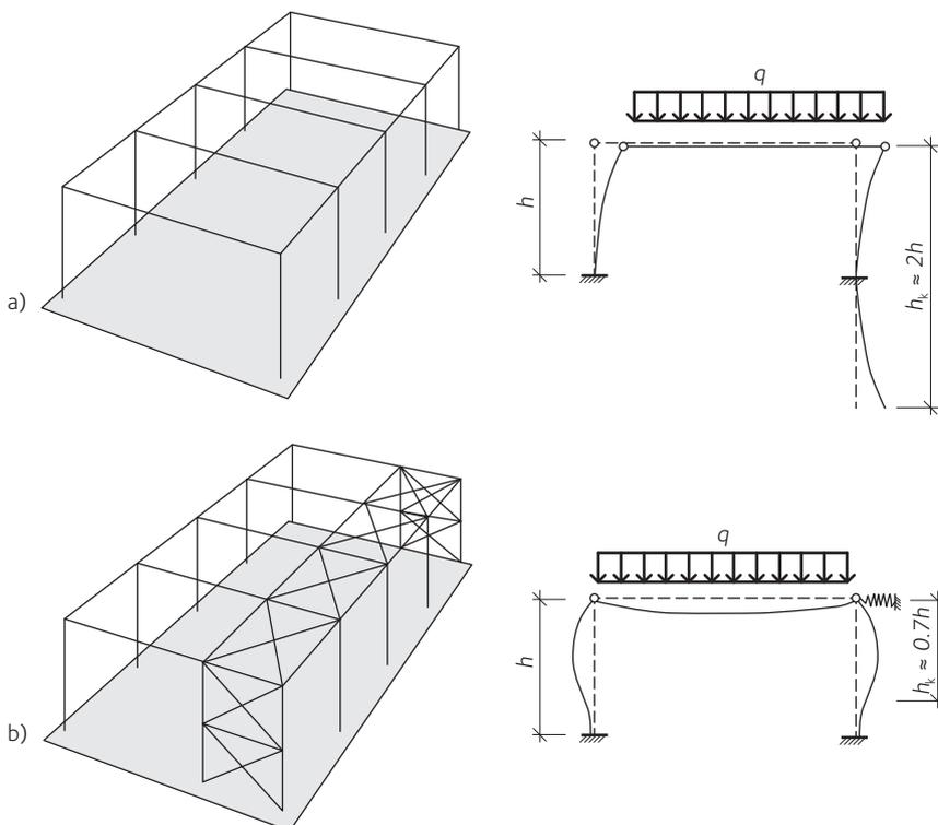
**Figure 13.11** Effect of longitudinal roof bracing on the buckling length of post-and-beam structures with columns rigidly fixed in the foundations
