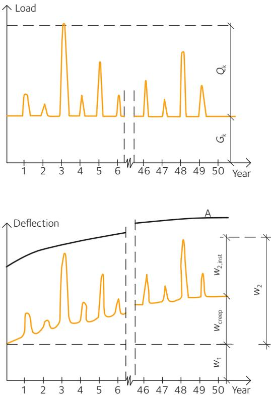
**Figure 6.1** Time variation, in principle, for deflection (lower figure) of a beam with permanent and variable loads according to the upper figure. Curve A shows the creep deflection if the beam were loaded with the characteristic loads  $G_k + Q_k$  during the whole period.
