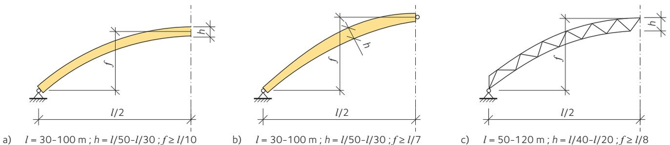
Figure 11.6 Preliminary design guidance for three different arch types
