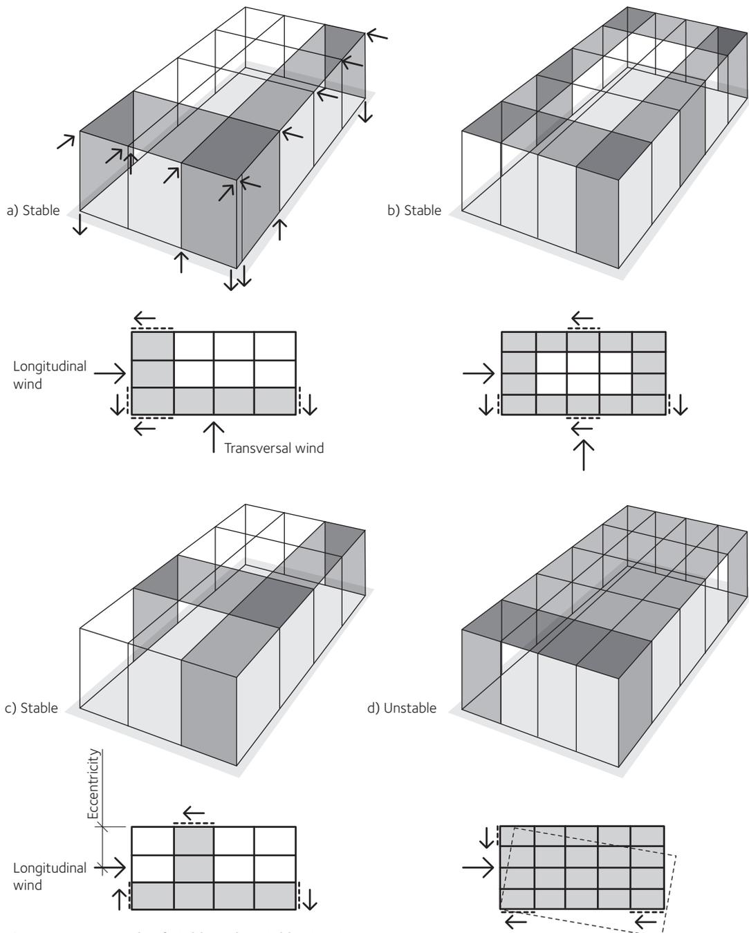
Figure 13.6 Example of stable and unstable structures
