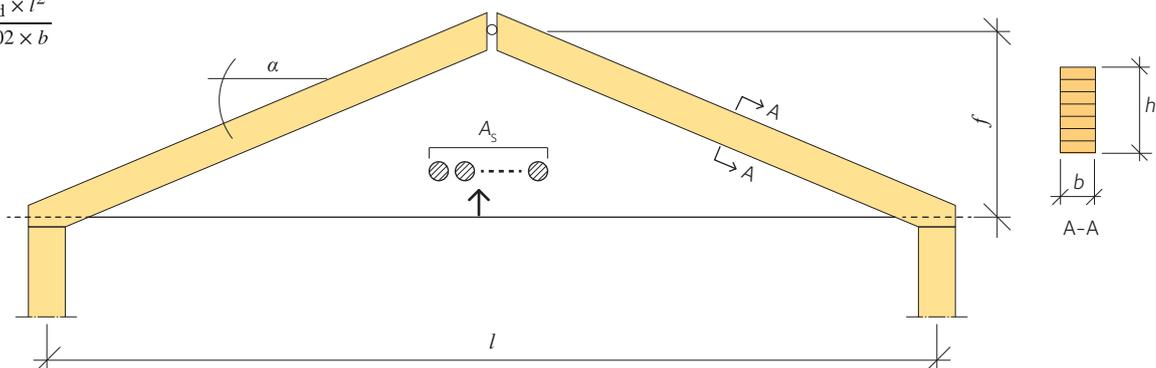
Figure 9.5 Typical three-hinged frame with steel tension tie
