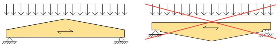
**Figure 7.4** Left: compression perpendicular to the grain occurs at the tapered edge.
