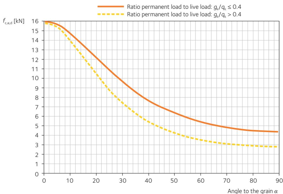
**Figure 4.12** Strength for glulam member loaded in compression at an angle  $\alpha$  to the grain
