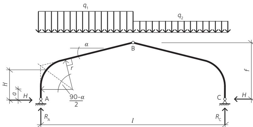
**Figure 10.2** Three-hinged frame with curved haunches, symbols
