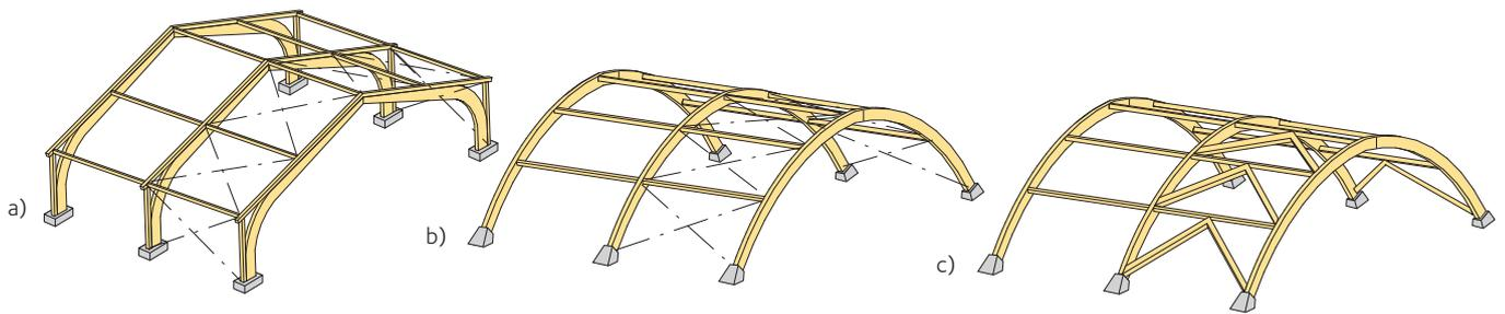
**Figure 13.35** Example of frame and arch bracing
