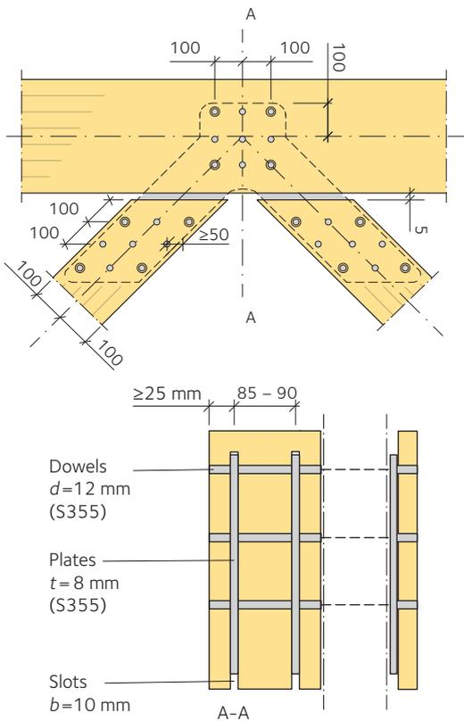
**Figure 8.17** Typical truss node used in Norway and Sweden with spacing indications. As many as 8 or 9 inset plates have been used for very heavy glulam trusses, but fewer inset plates across the width are sufficient for shorter spans.
