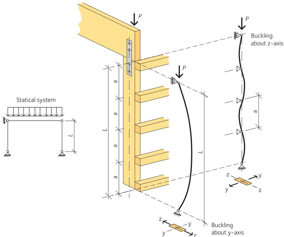
**Figure 4.19** Buckling of a timber column in an external wall
