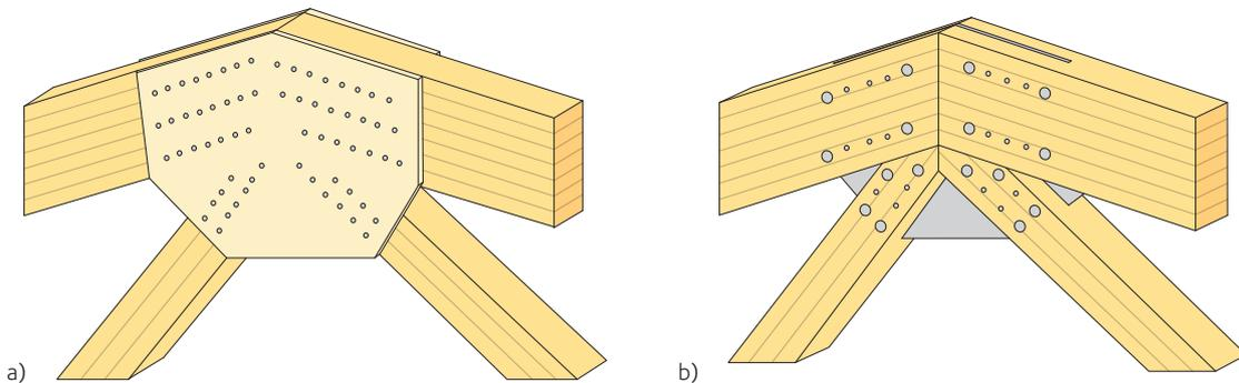
**Figure 8.20** Nodes at the ridge of pitched trusses
