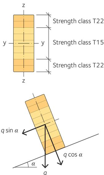
**Figure 1.10** Skew bending of a glulam beam
