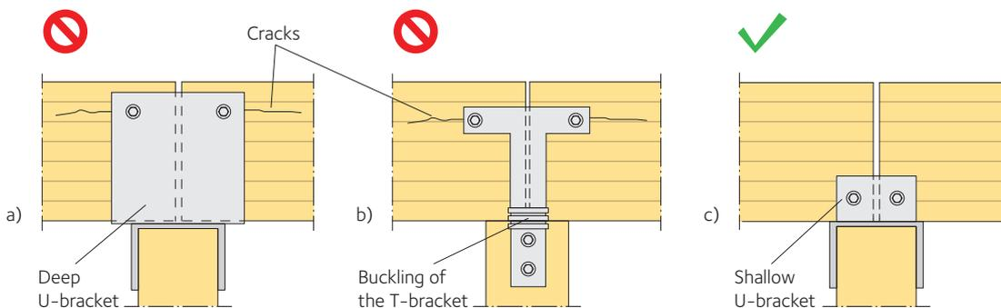
**Figure 15.2** Beam-to-column connections
