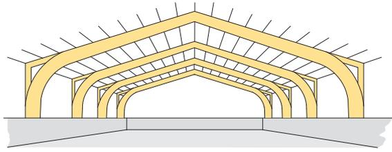
Figure 3.16 Portal frame with curved haunches
