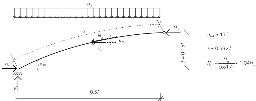
**Figure 11.14** Forces acting on one half of a three-hinged arch.  $\alpha_{1/4}$  is the angle between the axis of the arch and a horizontal line at the quarter point.  $s$  is the length of the semi-arch.  $N_{cr}$  is the Euler buckling load calculated at the quarter point of the arch.
