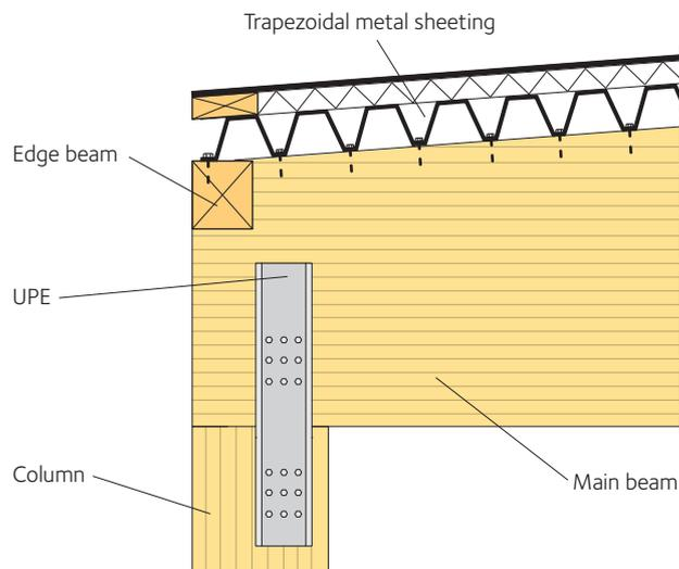
**Figure 13.34** Example of connections of trapezoidally corrugated metal sheeting to the main beam
