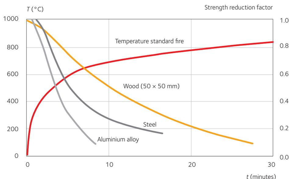
**Figure 16.1** Evolution of the mechanical properties of some building materials when exposed to a standard fire
