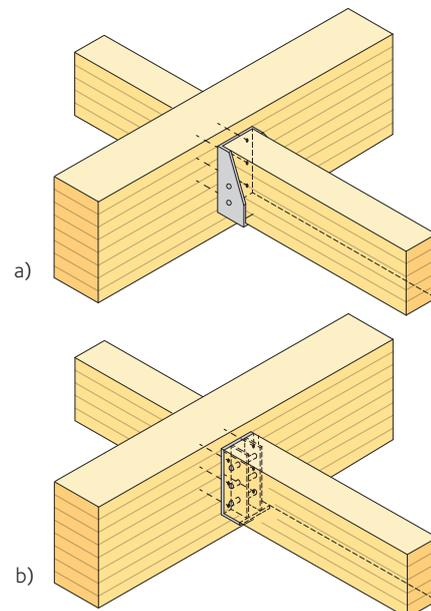
**Figure 14.24** Hangers side-mounted by means of screwing
