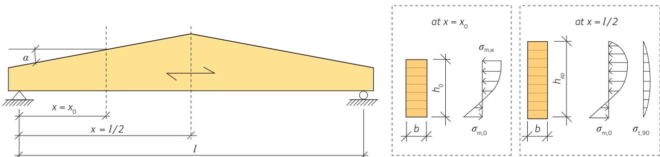
**Figure 7.8** Single tapered beam showing the real, nonlinear distribution of bending stress and perpendicular to grain stress at  $x = x_0$  and at mid-span
