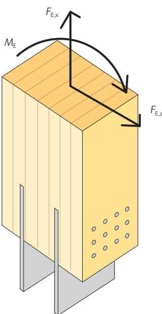
Figure 14.17 Slotted-in steel plates for fixed column base
