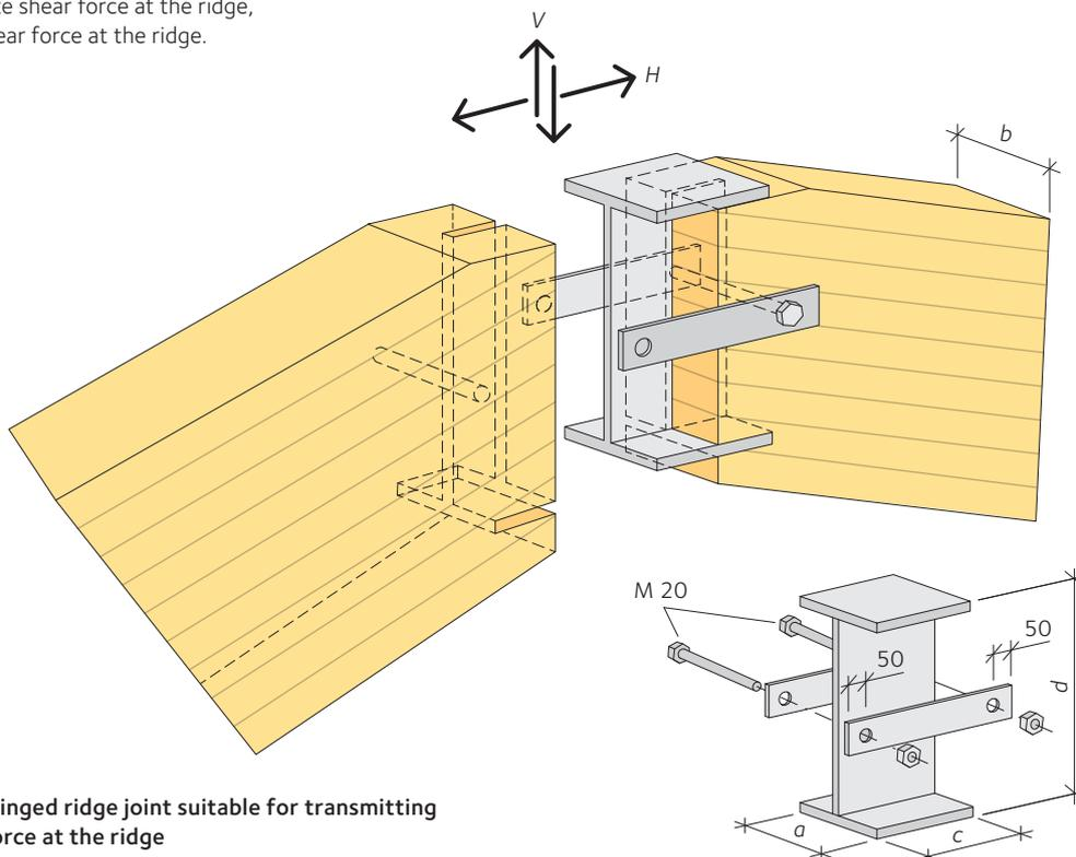
**Figure 9.9** Hinged ridge joint suitable for transmitting large shear force at the ridge
