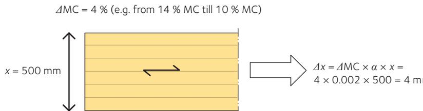
**Figure 14.3** Illustration of the magnitude of the shrinkage due to drying for a glulam beam. MC = moisture content.
