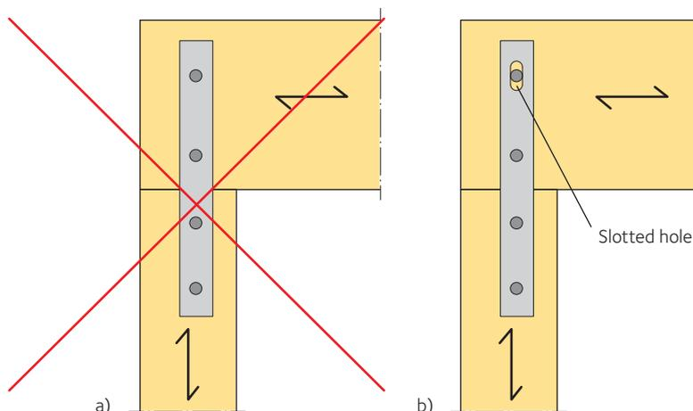
**Figure 14.4** a) A connection where movement perpendicular to the grain is constrained in the top beam
