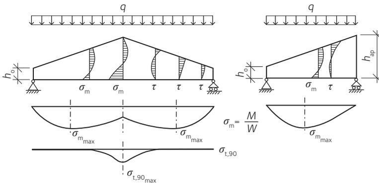
**Figure 7.2** Bending stresses ( $\sigma_m$ ), shear stresses ( $\tau$ ) and perpendicular to the grain tensile stresses ( $\sigma_{t,90}$ ) in double tapered beam (left) and single tapered beam (right)
