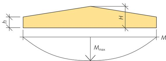
**Figure 3.5** The shape of a symmetrical double tapered beam approximates to the moment diagram of a beam simply supported and with uniform loading. It is therefore more economic in material than a constant-depth beam.
