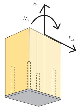
Figure 14.18 Fixed column base with bonded-in rods
