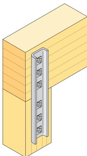
**Figure 14.28** U-shaped steel bars with running-through bolts
