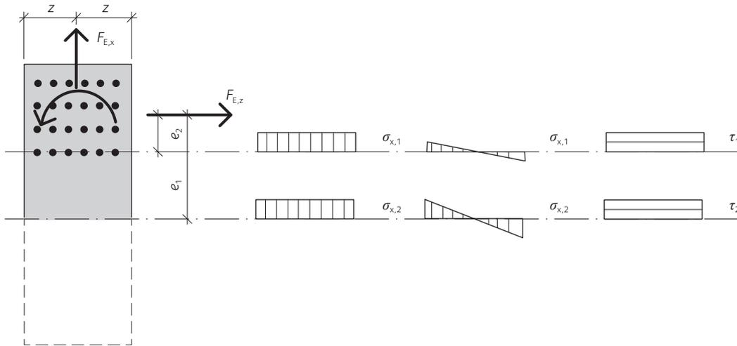
**Figure 14.27** Stress distribution in the steel plate
