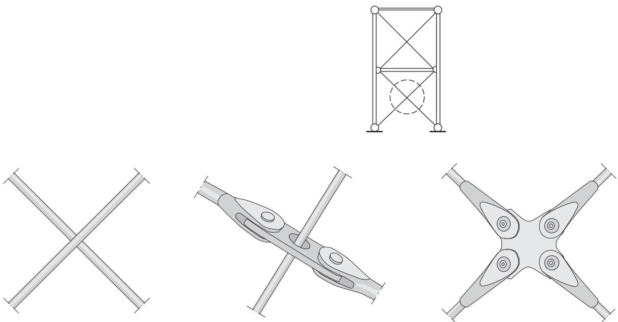
**Figure 13.22** Connection at the intersection between steel rods
