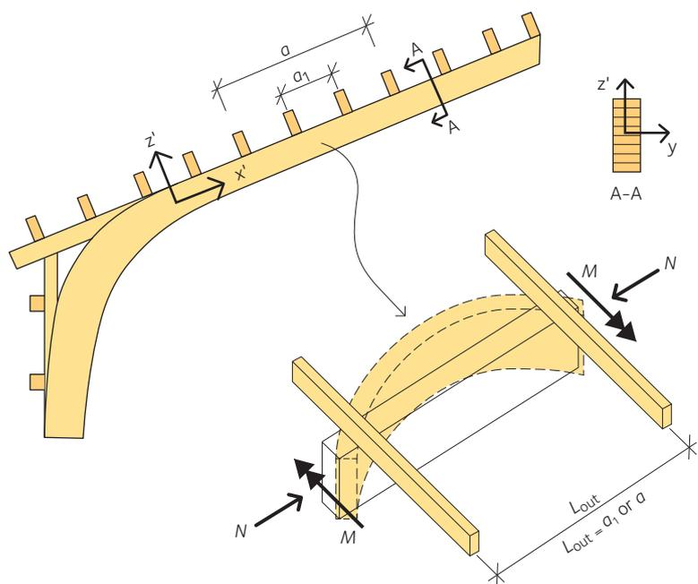
**Figure 10.5** Model for out-of-plane buckling check of the straight part of the frame. If the roof material is sufficiently stiff, the buckling length can be assumed to be equal to  $a_1$ . Otherwise, the buckling length should be assumed equal to  $a$ , see also figure 10.4, page 143.
