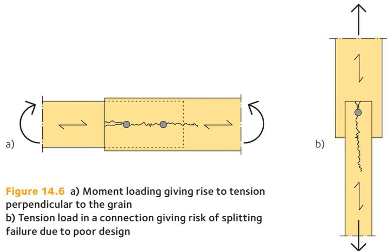
**Figure 14.6** a) Moment loading giving rise to tension perpendicular to the grain
