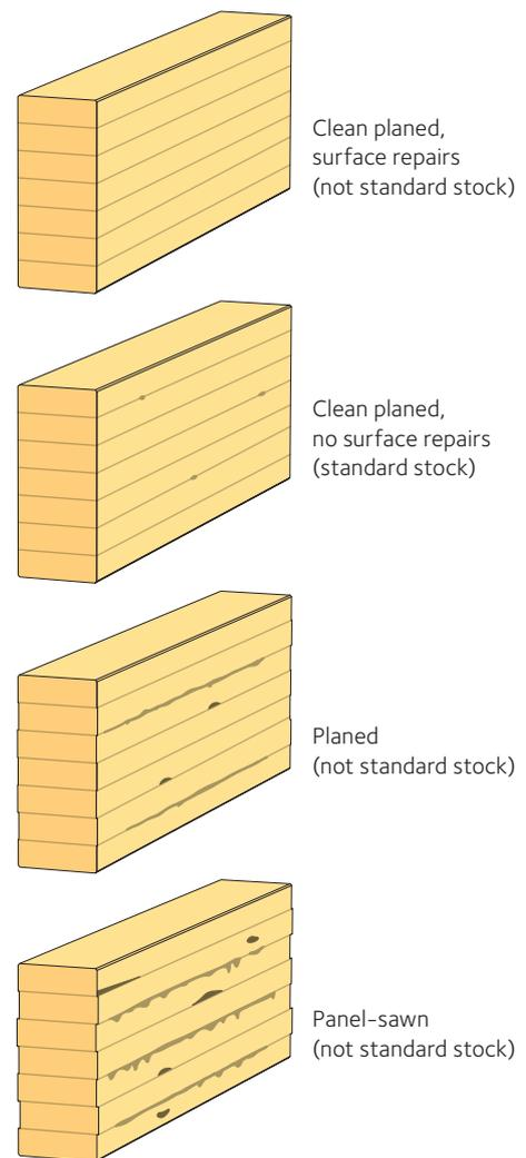
**Figure 1.12** Appearance grades, examples. From the bottom up: Panel-sawn, Planed (industrial appearance grade) and Clean planed, no surface repairs or Clean planed, surface repairs (architectural appearance grade), see also page 22-23 in *The Glulam Handbook Volume 1*.
