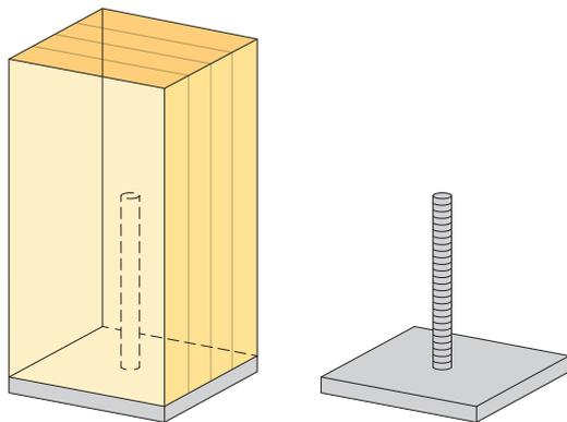
**Figure 14.12** Pinned column connection based on bonded-in rod
