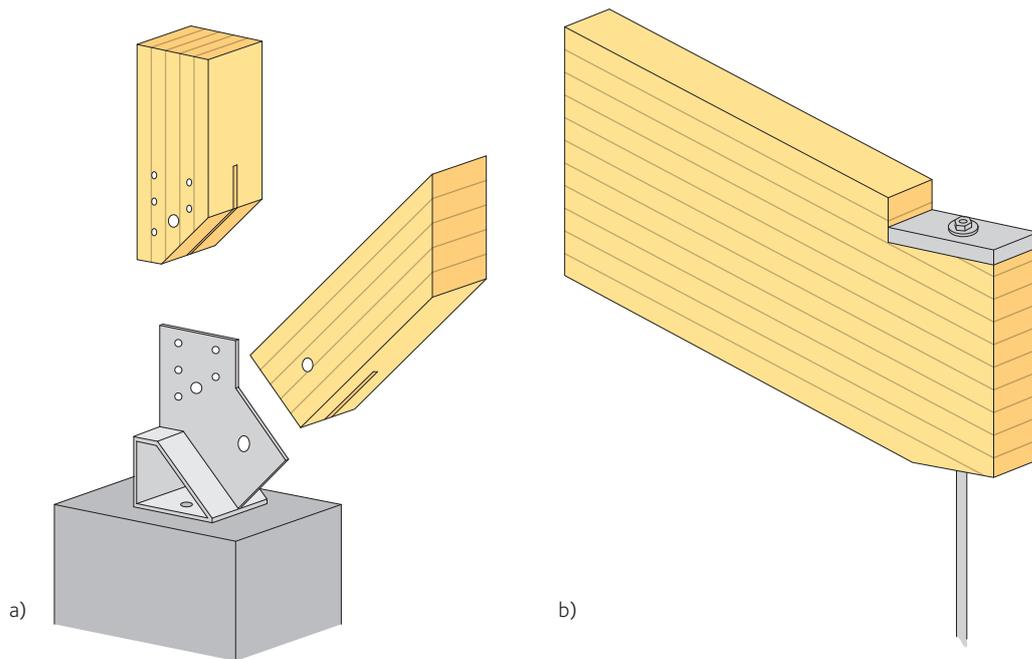
**Figure 10.17** Example of details in built-up frames
