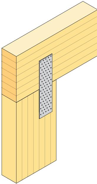
**Figure 14.25** Column top with externally mounted nail plates
