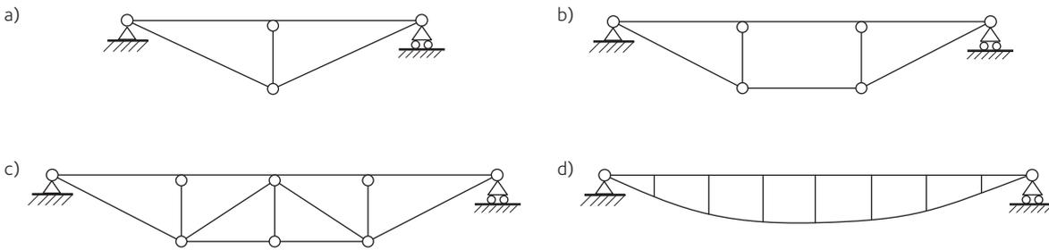
**Figure 3.11** a) – c) Trussed beams with different number of struts, d) fish belly beam.
