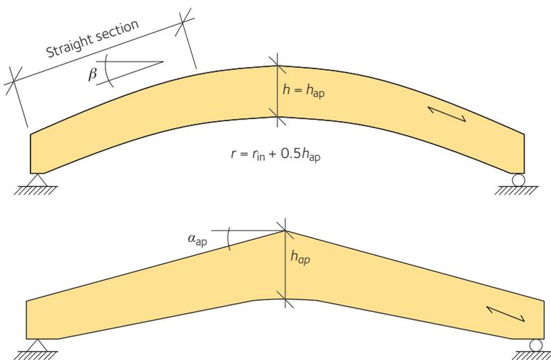
Figure 6.7 Curved beam (upper figure) and pitched cambered beam (lower figure)
