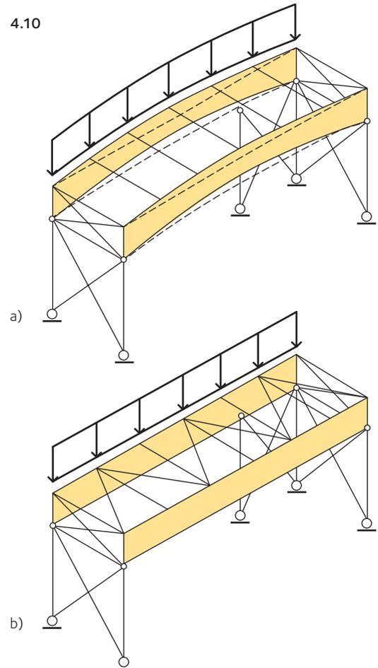
**Figure 4.4** Lateral bracing of slender beams
