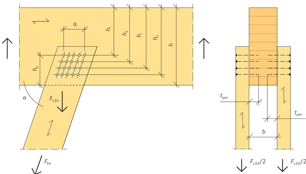
Figure 14.8 Notation used in design for splitting failure
