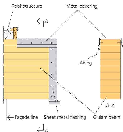
**Figure 1.13** An example of protection of an external cantilevering beam
