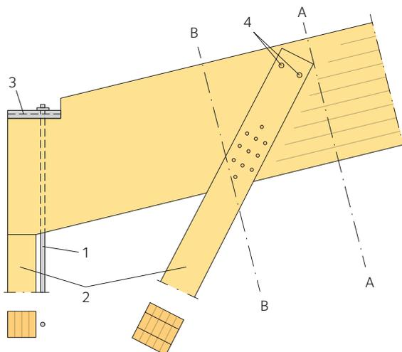
**Figure 10.13** Built-up haunch with bolted connection between rafter and inner leg
