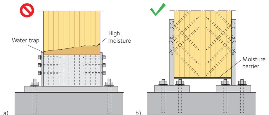
**Figure 15.11** Bracket at the base of a timber member (post, frame or arch)
