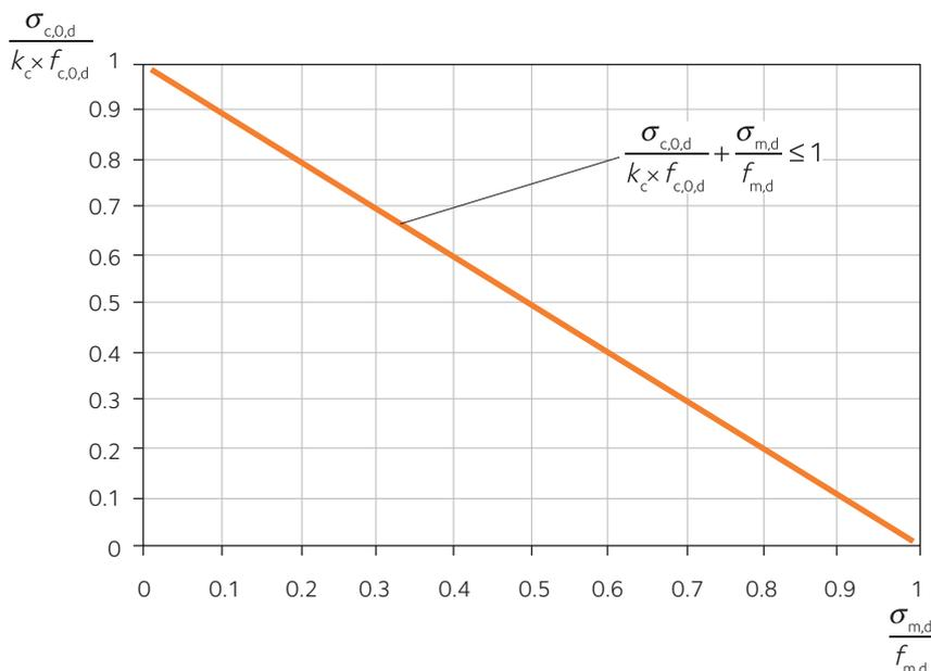
**Figure 4.22** Interaction diagram for combined bending and axial compression of a member about an axis,  $\lambda_{rel} > 0.3$  Elastic conditions. The index m,d is used as a generic and it refers to bending stress and bending strength respectively, caused by a bending moment either around “y” or around “z”. The index c,0,d refers to axial compression.
