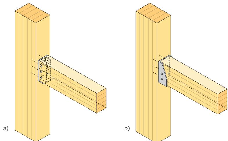
**Figure 14.20** Two different types of beam hangers
