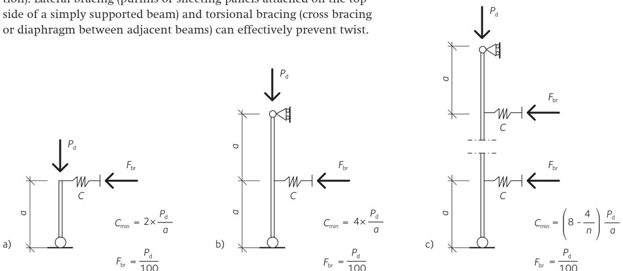
Figure 13.39 Recommended minimum brace stiffness,  $C_{min}$ , and corresponding brace force,  $F_{br}$ , where “n” is the number of brace points
