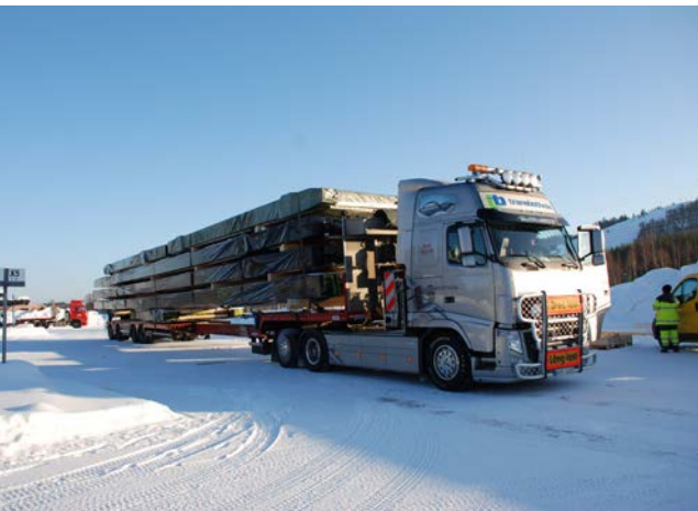
Glulam elements loaded onto a trailer for delivery to the construction site.
