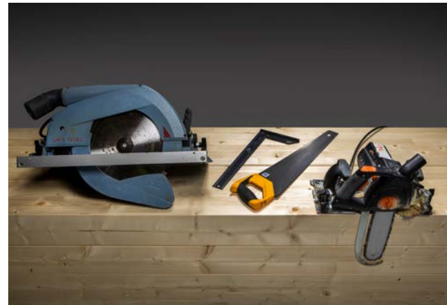
Examples of common power tools and hand tools for modifying glulam.
