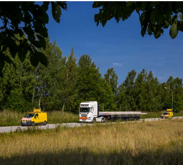
Transporting long glulam elements by semi-trailer. In this case, escort vehicles were required.
