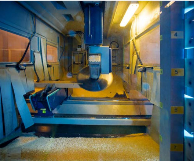
CNC machine at a glulam manufacturer.
