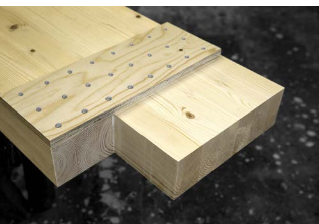
Example of notch and reinforcement with structural plywood that is screwed and glued to the glulam beam on both sides.
